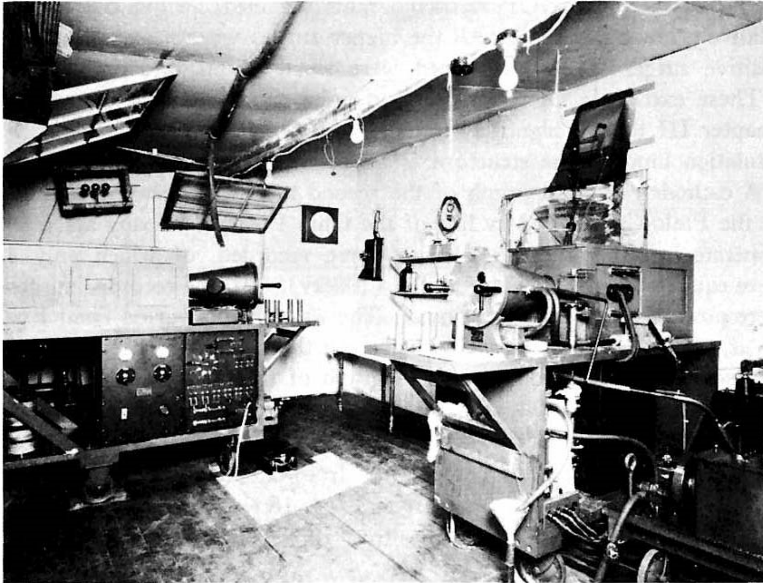
FIG. 5-8. Interior of oscillograph room in Wallenpaupack laboratory, 1929, showing two cathode-ray oscillographs, one for connection to transmission line and one for connection to antenna.
