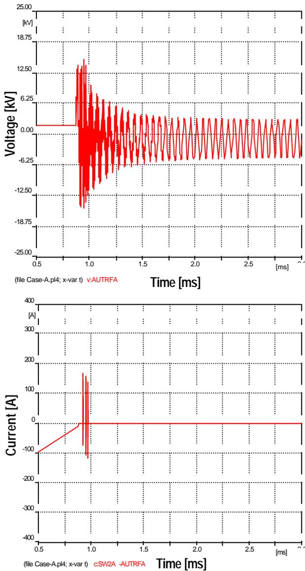
Fig. 4. a) Voltage at starting transformer, b) current through vacuum switch. Arc time = 0.8 ms
