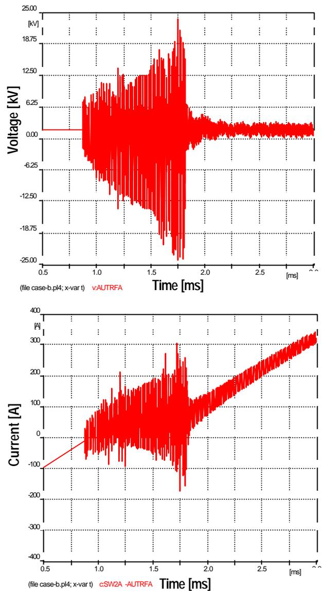
Fig. 5. a) Voltage at starting transformer, b) current through vacuum switch. Arc time = 0.25 ms
