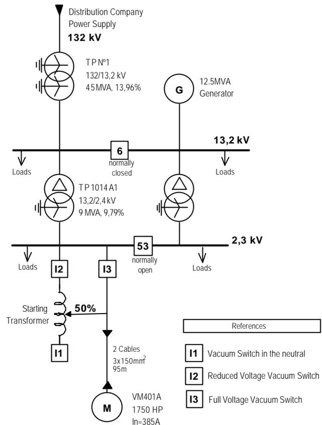
Fig. 1. Single-wire of the network to simulate.
