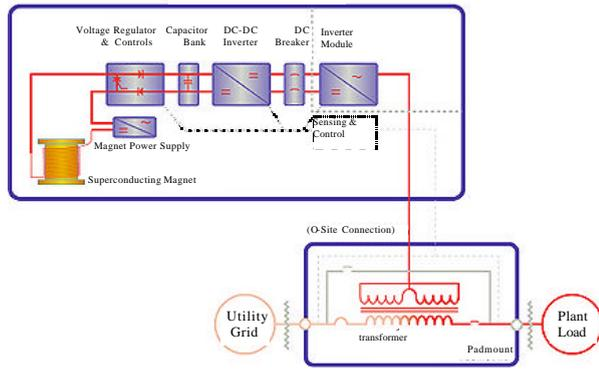
Figure 1 – Typical PQ-VR functional block diagram
