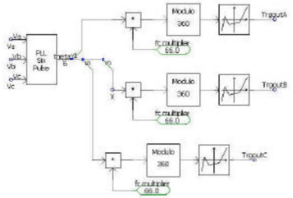
Figure 6 – Generating the 4kHz sine-triangle carrier signals.
