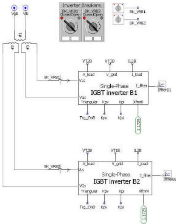
Figure 4 – PQ-VR inverter modules connected in series to a distribution system.
