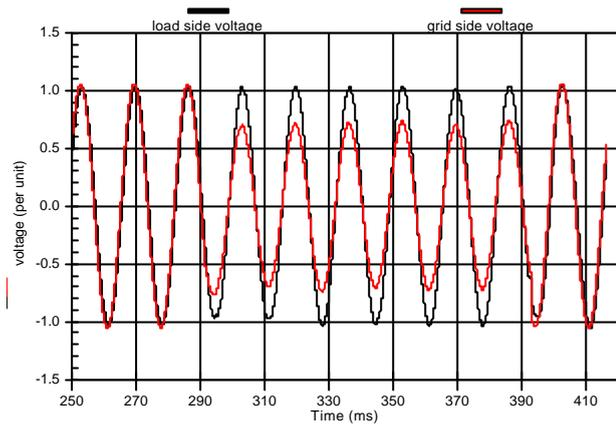
Figure 11 – PQ-VR in carryover mode. The voltage sag is at the grid side. The load side voltage remains at 1.0 per-unit since the PQ-VR successfully holds the voltage.
