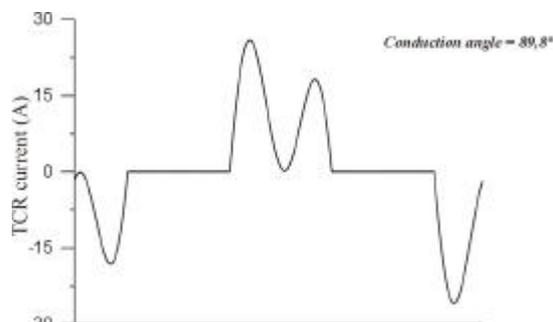
Fig. 8 – Steady-state reactor current
