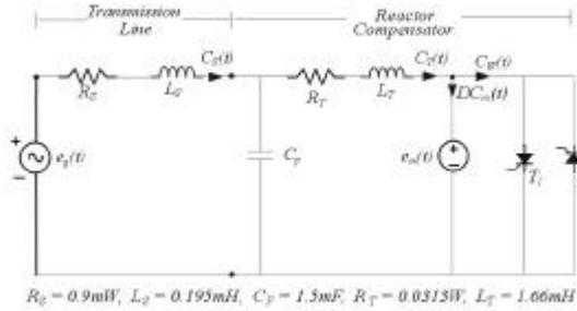
Fig. 1 – Single-phase Static VAR System
