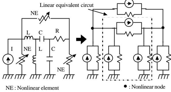
Fig. 3 Equivalent circuit for a nonlinear circuit
