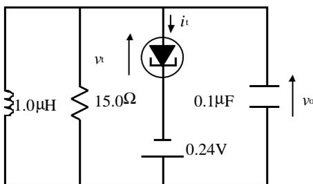
Fig. 6 Oscillator circuit using a tunnel diode
