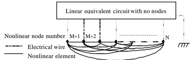
Fig. 4 Relation between LU decomposition and a nonlinear equivalent circuit
