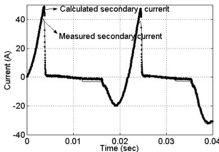
Fig. 9. Secondary current measured and calculated in CT 2.
