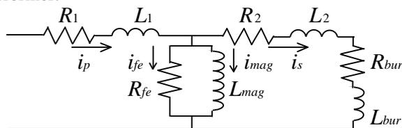
Fig. 1. Equivalent circuit of a transformer.
