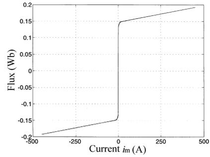
Fig. 4: Flux-current curve of transformer 2.
