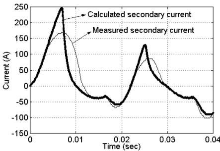
Fig. 8. Secondary current measured and calculated in CT 1.
