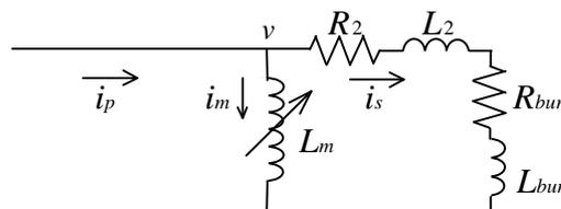
Fig. 2. Simplified equivalent circuit of the a current transformer.
