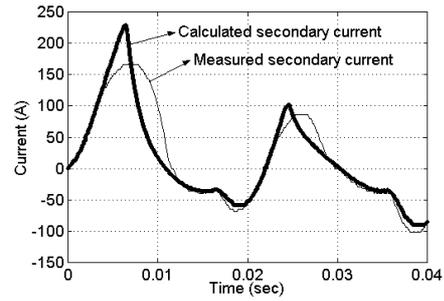
Fig. 10. CT 1 considering a leakage reactance of  $0.1 \Omega$  to 50 Hz
