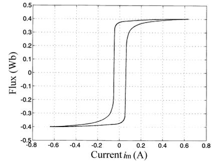
Fig. 5: Flux-current curve of transformer 1, low current applied.
