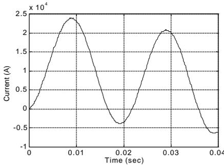
Fig. 7. Primary current measured in the test (CT 2).
