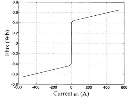
Fig. 3: Flux-current curve of transformer 1.
