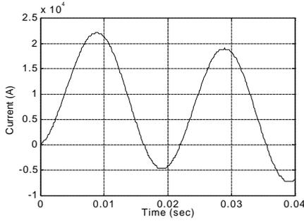
Fig. 6. Primary current measured in the test (CT 1).
