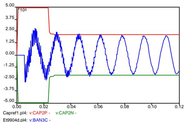
Figure 4 – Bank 3 – Energizing TOV – 2 daily switching – Inductor losses represented.
