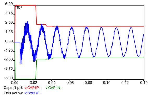
Figure 3 – Bank 3 – Energizing TOV – 1 daily switching – Inductor losses represented.
