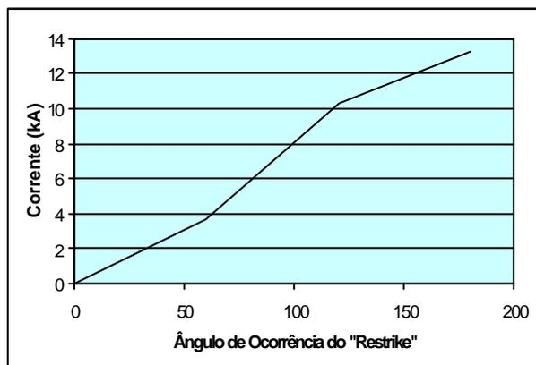
Figure 7 – First peak current versus restrike angle.
