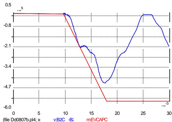
Figure 6 – Bank 2 capacitive current opening TRV, sound phase of double line to ground fault
