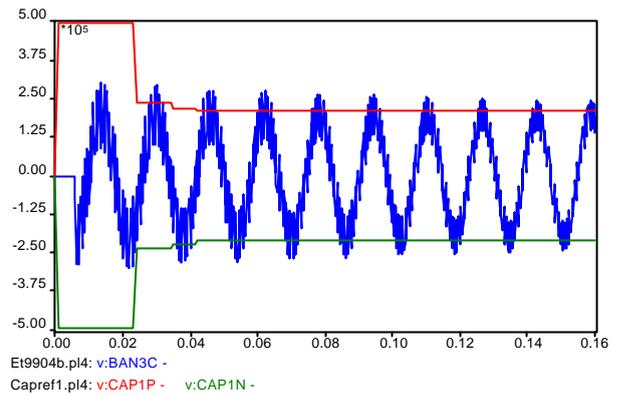
Figure 1 – Bank 3 – Energizing TOV – 1 daily switching – No inductor losses represented.
