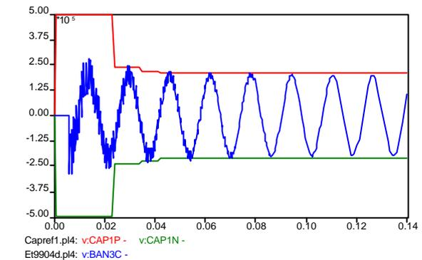
Figure 3 – Bank 3 – Energizing TOV – 1 daily switching – Inductor losses represented.
