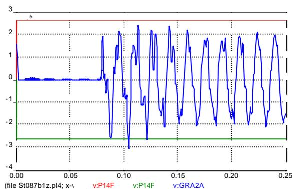
Fig. 5 – Temporary overvoltages in the substation, due to the transformer saturation.
