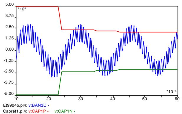
Figure 2 – Bank 3 – Energizing TOV – 1 daily switching – No inductor losses represented.
