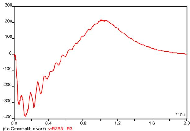
Figure 8 – Lightning overvoltages across the inductor.
