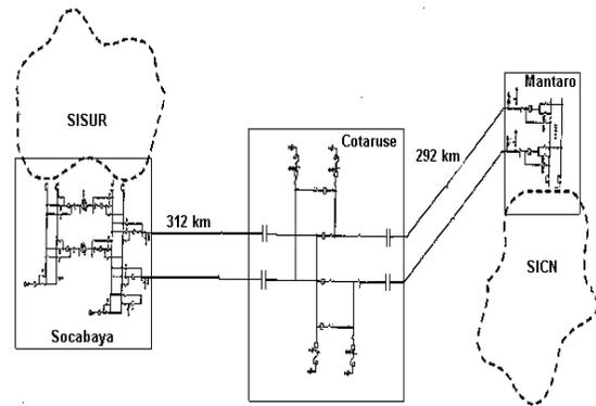
Transient recovery voltage on the 220kV breakers, temporary and switching overvoltages, energy stresses on MOV and implementation of protection and automatic switching schemes. The electromagnetic transient studies were performed with DCG-EMTP.
