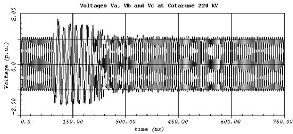
**FIG-III.1a: Voltages at the Cotaruse 220 kV Bus bar**
