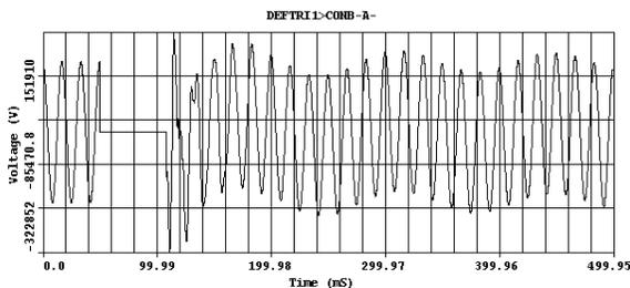
**FIG.V-II Voltage after fault clearing at Cotarus**
