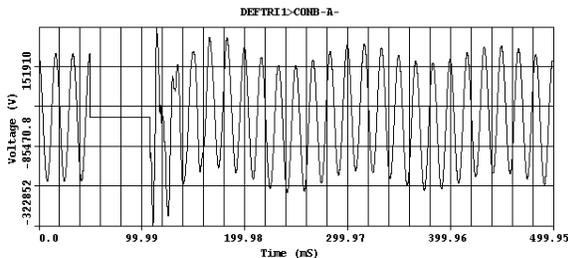
**FIG.V-II Voltage after fault clearing at Cotarus**
