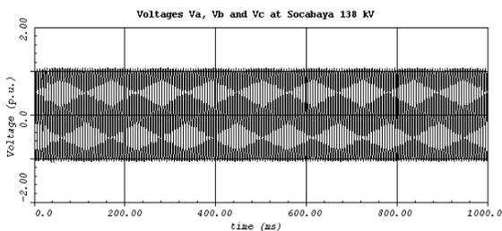
FIG-III.3c Voltages at Socabaya 138 kV after Transformer Energization ( with 400 ohms resistance)
