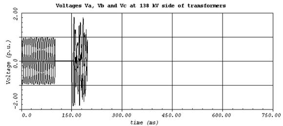
**FIG-III.2.1d Voltages at 138 kV Side of Transformers**
