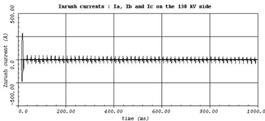
FIG-III.2.3c Inrush Current on 138 kV side
