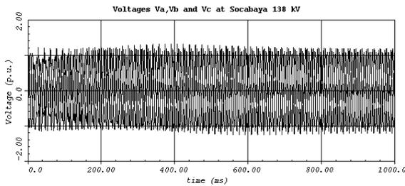
FIG-III.3.a Voltages at Socabaya 138 kV after Transformer Energization ( no insertion resistance)
