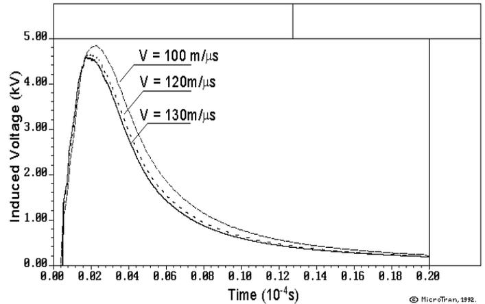
Fig 3 Induced voltage for the most usual velocities (100, 120 and 130m/ $\mu$ s) – Flash n<sup>o</sup> 9305
