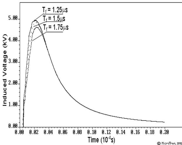
Fig.4. Effects of front time – Flash n<sup>o</sup> 9305
