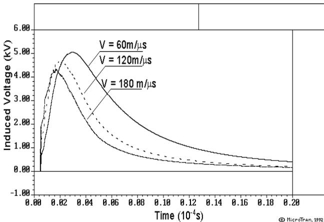
Fig. 2. Induced voltage as a function of velocity, Flash n<sup>o</sup> 9305
