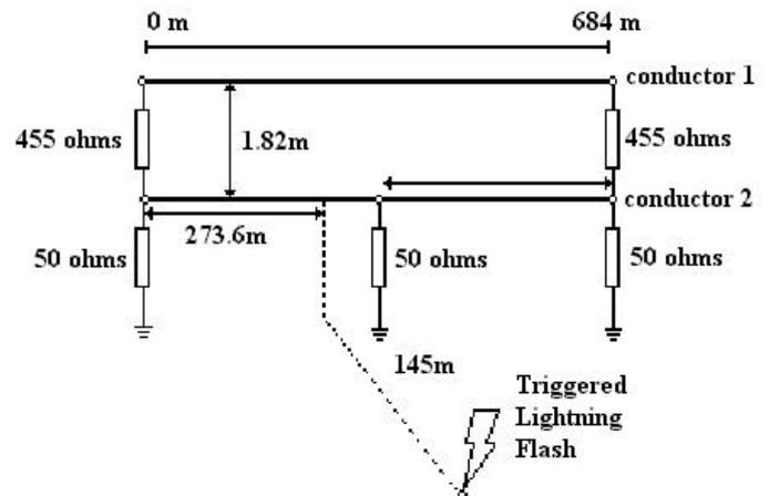
Fig. 1. Phase conductor 1 and neutral conductor 2, and discharge configuration.
