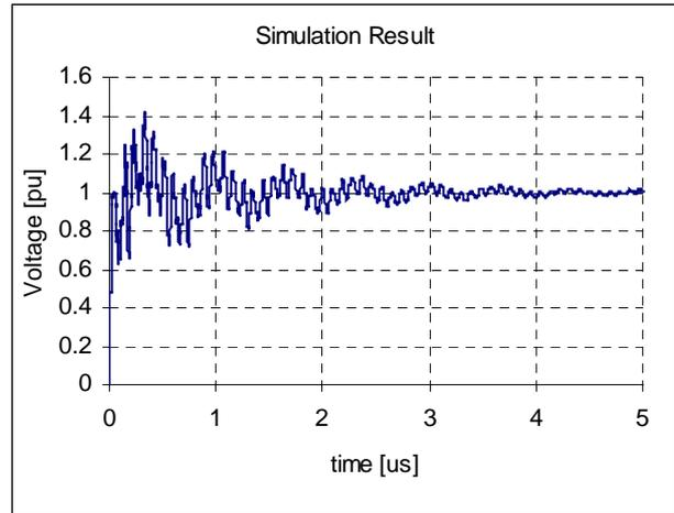
Fig. 4. VFT EMTP simulations.
