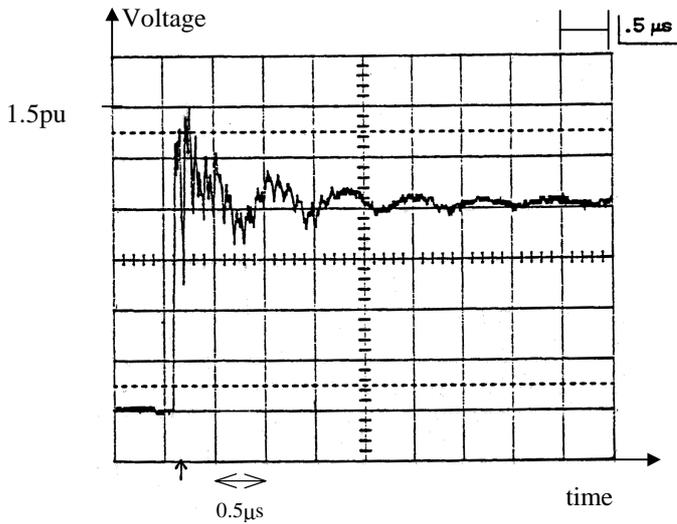
Fig. 2. Measurement of Very fast transient for test duty 1
