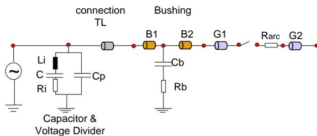
Fig. 3. Equivalent circuit for simulation
