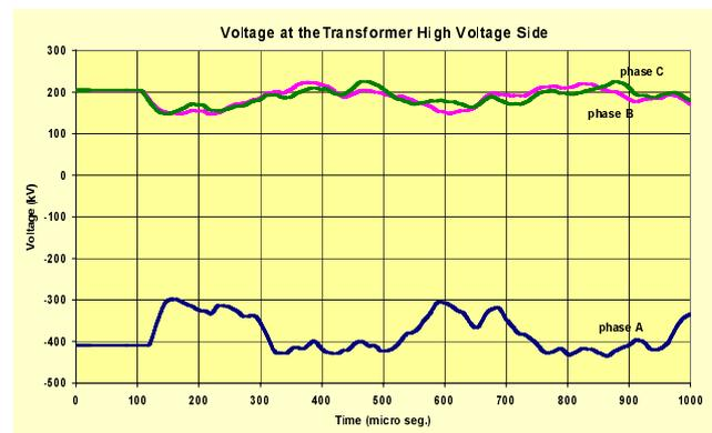
Fig. 8. VFT Overvoltage at the low voltage side of the transformer T2
