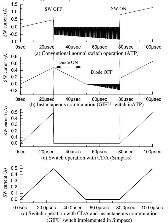
Fig. 5 Chopper circuit operation in discontinuous current mode
