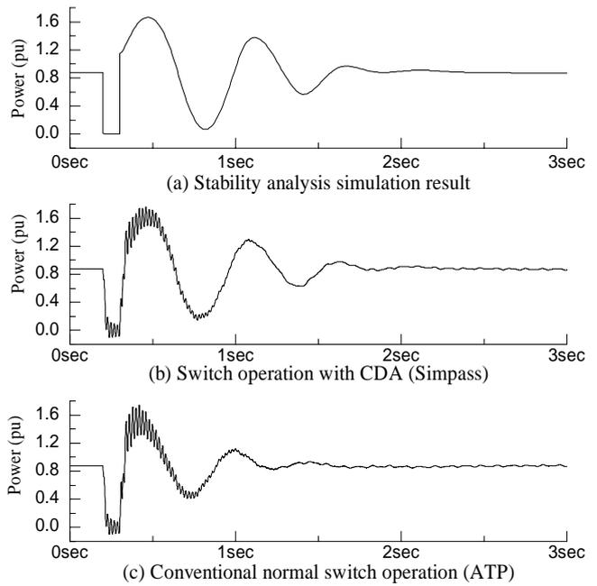
Fig. 9 Generator output power
