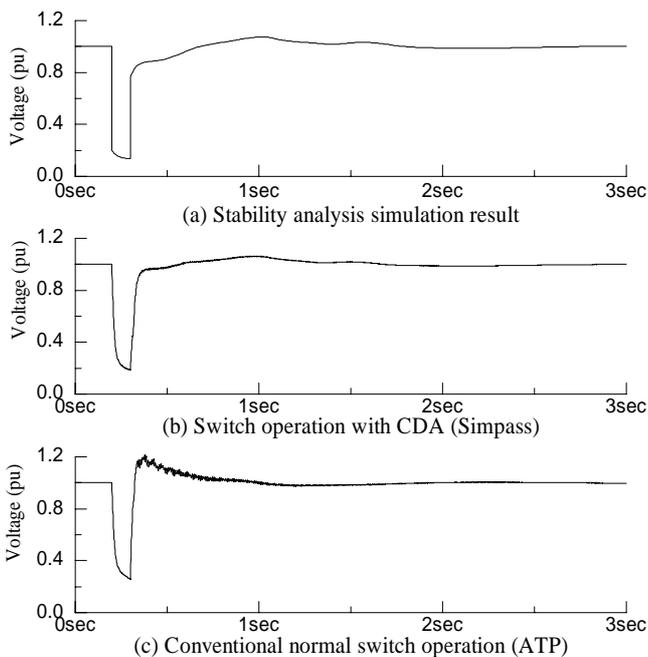
Fig. 8 RMS value of ac bus voltage at generator terminal
