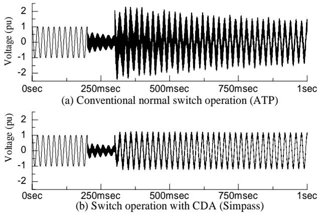
Fig. 7 AC voltage at the generator terminal (Phase A)
