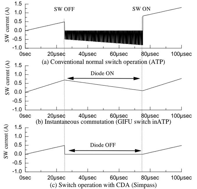
Fig. 4 Chopper circuit operation in continuous current mode
