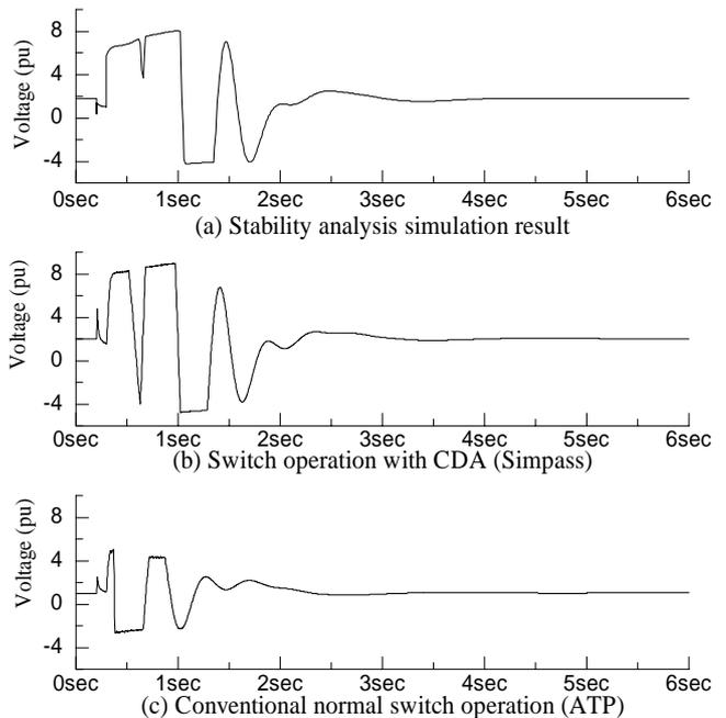
Fig. 10 Exciter voltage of generator (Thyristor type)
