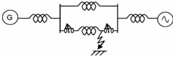
Fig. 6 Studied one machine and infinite bus power system model
