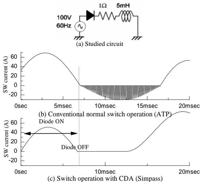
Fig. 2 Half-wave rectification circuit
