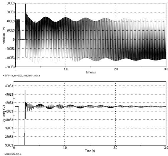
Fig. 4 Voltage Waveform (top) and Phasor Amplitude (bottom) at Ancoa for a 525 kV Busbar Fault with One Shunt Reactor 500-220 kV Transformer Out of Service.
