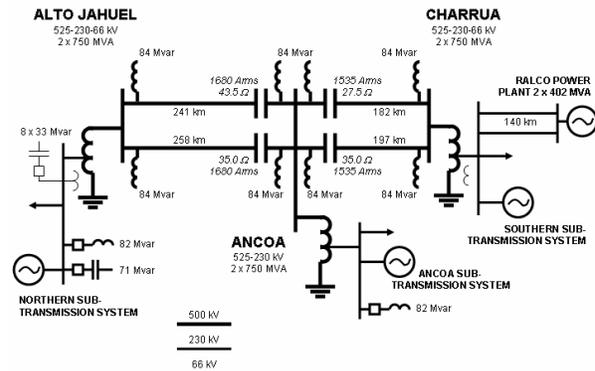
Fig. 1 The Chilean 500-kV Series-Compensated Transmission System
