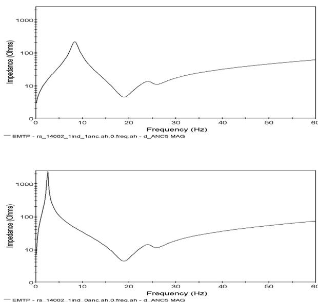
Fig. 3 Frequency Response at Ancoa 525 kV with One 525 kV Shunt Reactor
