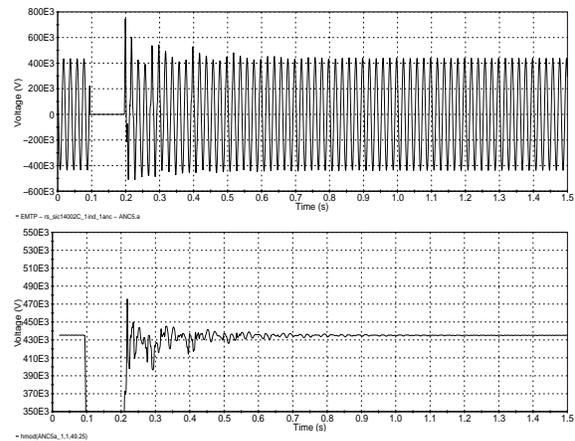
Fig 6 Voltage Waveform and Phasor Amplitude at Ancoa for a 525 kV Busbar Fault – 525-230 kV Transformer In Service.
