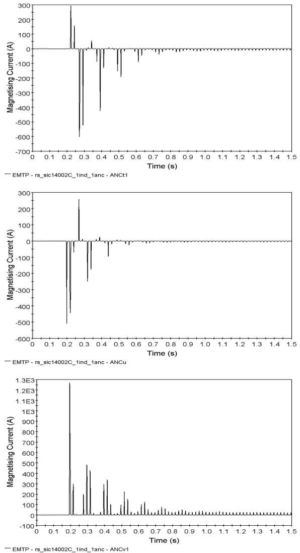
Fig. 5 Inrush Currents in phases a, b and c of the 500-220 kV Transformer at Ancoa Following a 3φ fault
