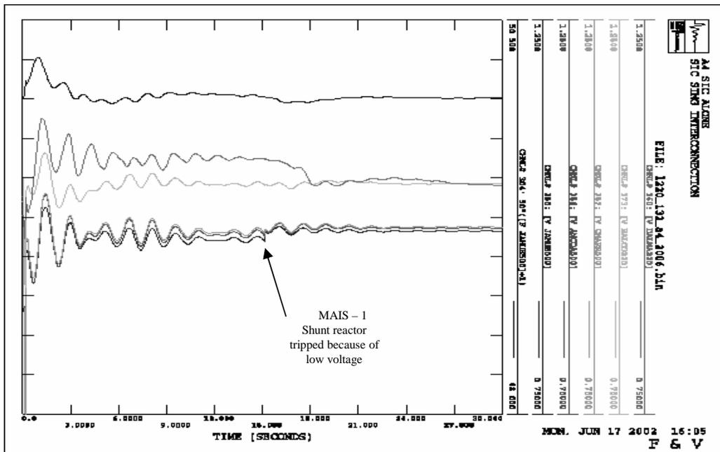
Fig 2: 1L-G Fault at Ancoa 525 kV with the Loss of Ancoa – Alto Jahuel 525 kV Line
