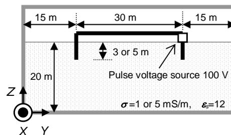
Fig. 7 Two buried vertical thin wires connected by an overhead horizontal wire to be analyzed by the FDTD method
