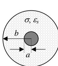
Fig. 1 Cross section of a thin wire surrounded by a cylindrical sheath
