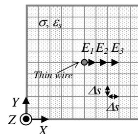
Fig. 2 Electric fields around a thin wire in a rectangular sheath to be used for an FDTD analysis
