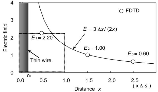
Fig. 6 Radial electric fields as a function of distance from the thin wire [7] (The value of electric field is normalized so that  $E_2$  should be unity)
