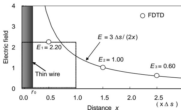
Fig. 6 Radial electric fields as a function of distance from the thin wire [7] (The value of electric field is normalized so that  $E_2$  should be unity)
