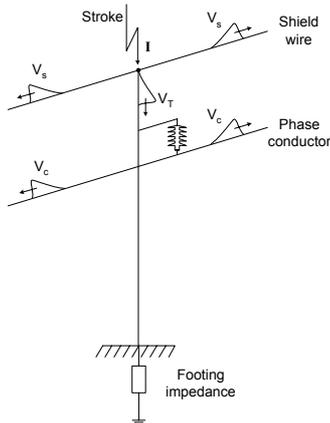
Fig. 1. Lightning stroke to a transmission line.
