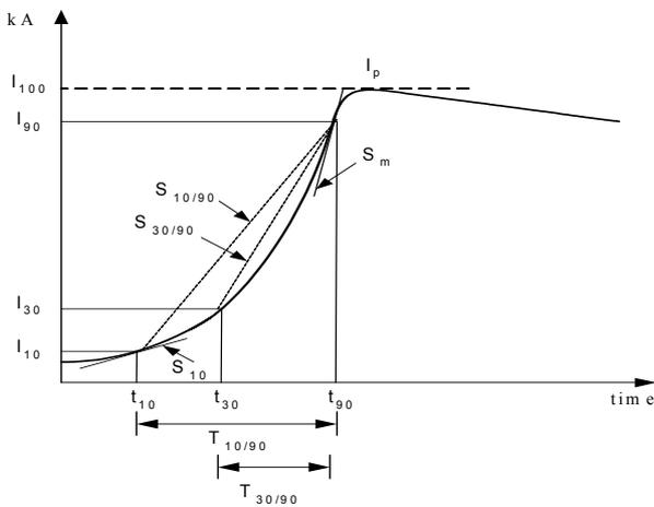
Fig. 3. Parameters of a return stroke – Concave waveform.
