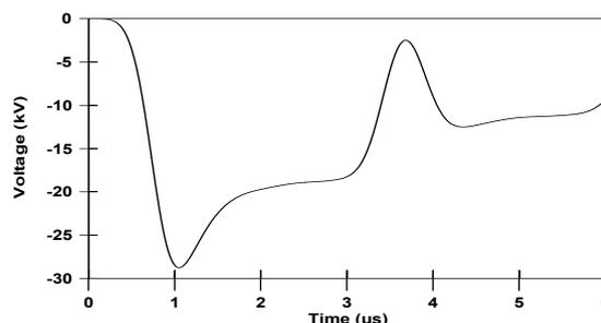
Fig. 6. Backflash insulator stress – Outer phase ( $I_{max} = 1$  kA,  $t_f = 1$   $\mu$ s,  $R_{tower} = 20$   $\Omega$ )
