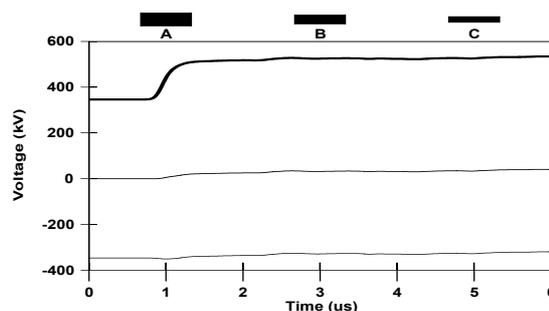
Fig. 8. Shielding failure insulator stress (1 kA,  $t_{max} = 1$   $\mu$ s). Phase voltages are included in the simulation.
