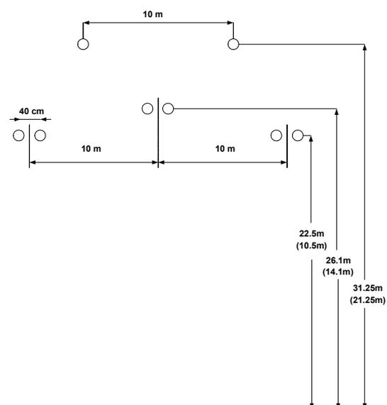
Fig. 2. 400 kV line configuration (Values between parenthesis are midspan heights).
