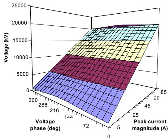
Fig. 9. Shielding failure. Insulator stress as a function of the peak current and the voltage angle ( $t_f = 1 \mu s$ ).
