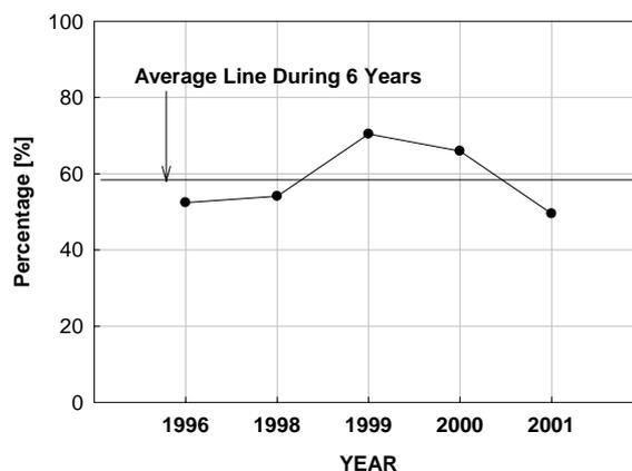
Fig. 4 The detection rate of LPATS by the comparison with real failures in the power system
