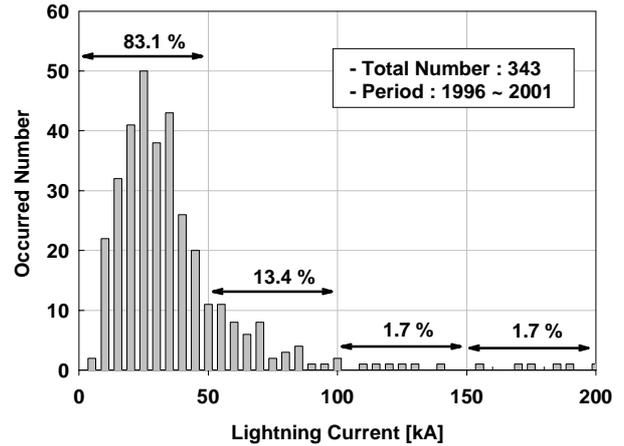
Fig. 3 The amplitude distribution of lightning current, which caused to the outages
