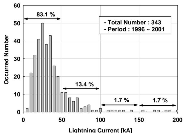
Fig. 3 The amplitude distribution of lightning current, which caused to the outages
