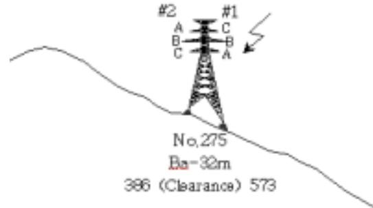
Fig. 8 The tower configuration and the SFFOR concept in 765 kV line
