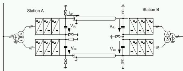
Fig. 1 Typical circuit diagram of a bipolar HVDC Transmission System
