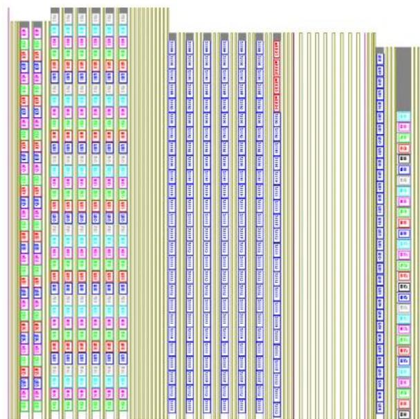
FIG. A.2 A Cross-section of the winding with few sections of the winding subdivided in the axial and radial directions. Each subdivision was analytically modeled as an inductance-capacitance network. This figure is only for illustrative purpose of the modeling concept and actual number of sub-divisions was far higher.
