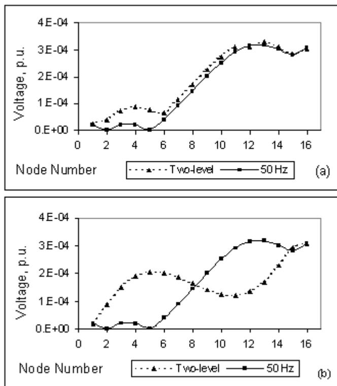
Fig. 7. Voltage distribution across Tertiary windings (TWs) under the influence of two-level and 50 Hz wave excitation. (a) TW1 (b) TW2.
