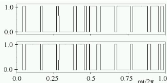
Fig. 3 Typical voltage output waveform of a two-level VSC system
