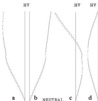
Fig 4 Voltage distribution of HV winding under two level voltage waveform excitation at different time instants.
