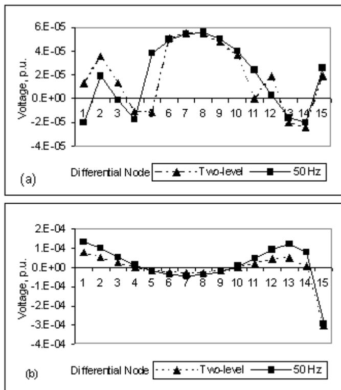
Fig. 9. Differential Voltage distribution across Tertiary windings under the influence of two-level and 50 Hz wave excitation. (a) TW1 (b) TW2.
