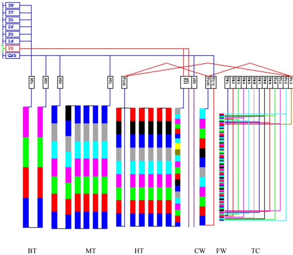
FIG. A.1 Schematic Diagram of the transformer
