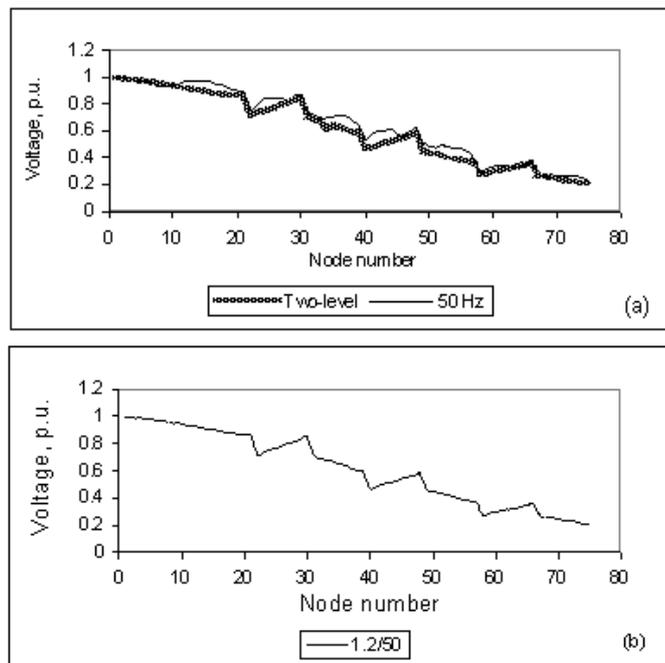
Fig. 6. Voltage distribution across HV winding under the influence of (a) two-level and 50 Hz (b) 1.2/50 impulse wave excitation.
