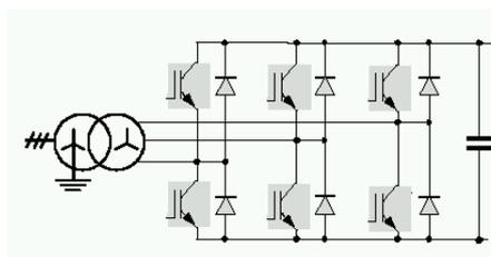
Fig. 2: Equivalent circuit of a 6 pulse IGBTs based 2 Level VSC
