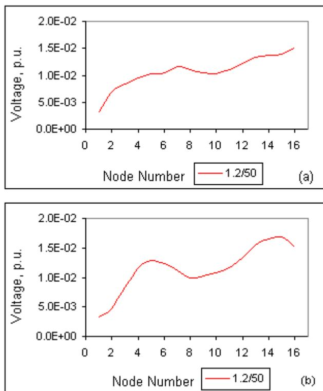
Fig. 8. Voltage distribution across Tertiary windings (TWs) under the influence of 1.2/50 impulse excitation. (a) TW1 (b) TW2.
