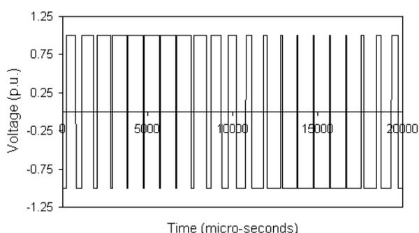
Fig. 5 Analytically generated two-level VSC waveform
