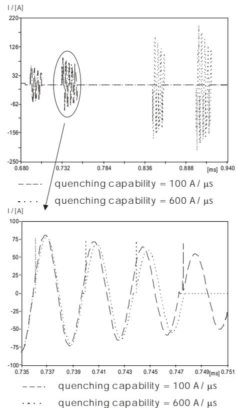
Figure 10 The current pattern with variation of the quenching capability
