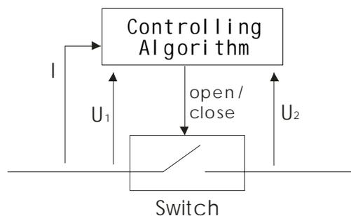
Figure 1 Model of Vacuum Circuit Breaker
