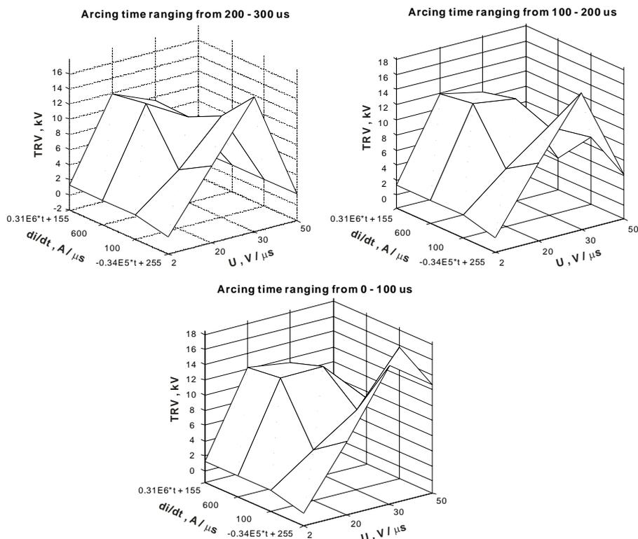
Figure 11 Escalation voltages as a function of the breaker model characteristics
