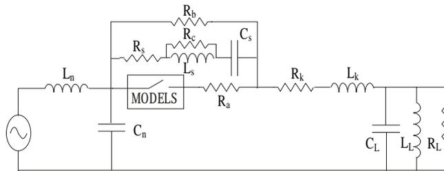
Figure 2 Helmer's circuit
