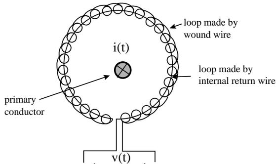
Figure 7. Rogowski Coil with the Return wire Through the Winding Center
