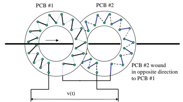
Figure 8. Principle of the PCB Rogowski Coil Design
