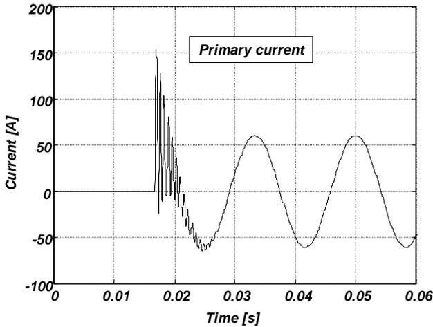
Figure 19. Capacitor Energizing (primary current)
