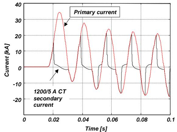
Figure 18. Current Transformer Transient Response to Asymmetric Faults
