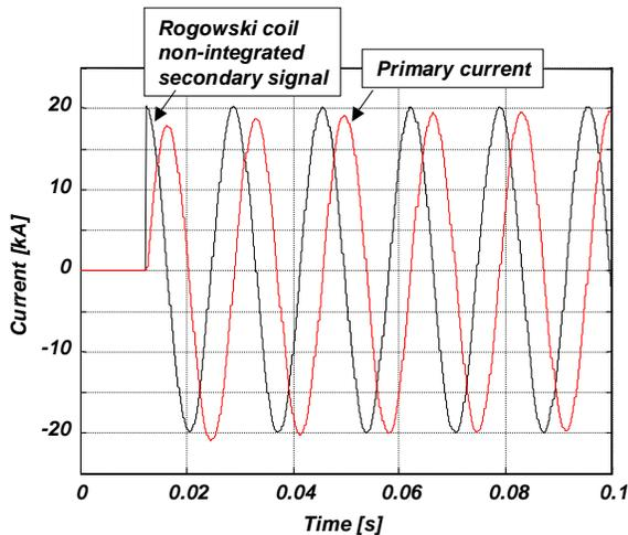
Figure 15. RC Transient Response to Symmetric Faults (non-integrated RC secondary signal)
