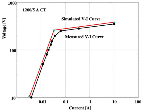
Figure 4. 1200/5 A Current Transformer V-I Curve
