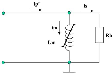
Figure 3. Current Transformer Modeling for the Relay Transient Studies
