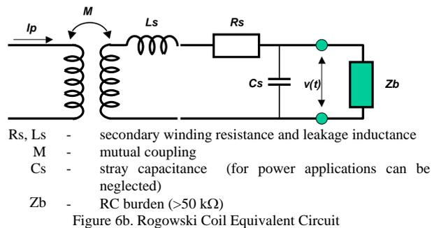
Figure 6b. Rogowski Coil Equivalent Circuit
