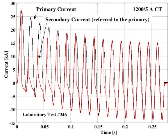
Figure 5. 1200/5 A Current Transformer Transient Performance
