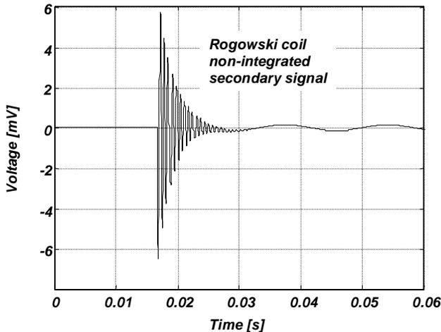
Figure 20. RC Transient Response to Capacitor Energizing (non-integrated RC secondary signal)
