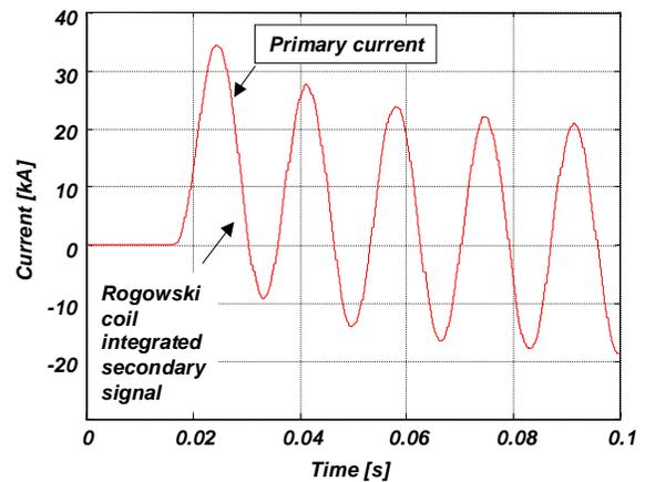
Figure 17. RC Transient Response to Asymmetric Faults (integrated RC secondary signal overlaps the primary current waveform)
