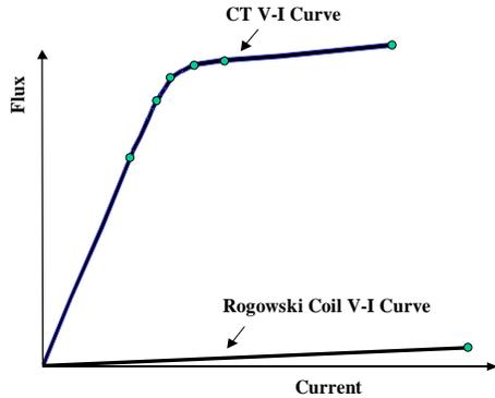
Figure 13b. Rogowski Coil and Current Transformer Flux-Current Characteristics
