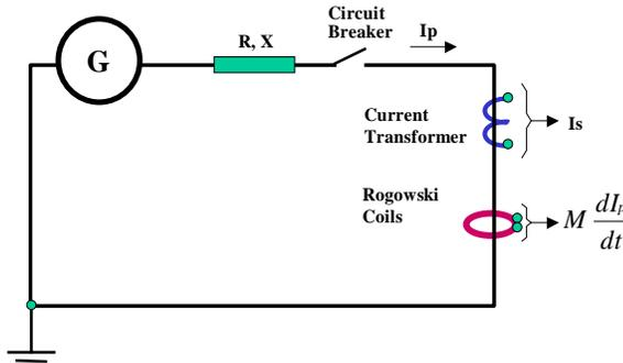
Figure 14. ATP Model for Simulation of CT and RC Transient Responses
