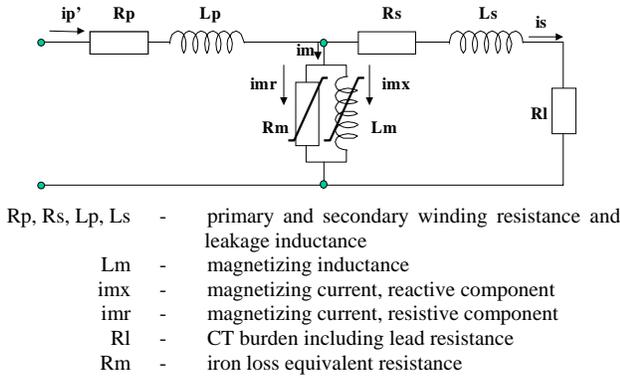
Figure 2. Current Transformer Equivalent Circuit
