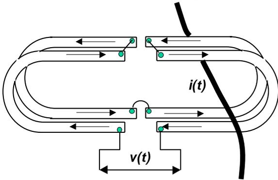
Figure 10. Principle of the Split-Core Style PCB Rogowski Coil Design
