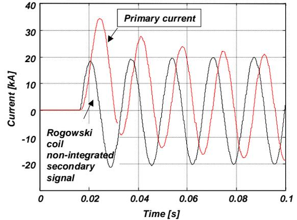
Figure 16. RC Transient Response to Asymmetric Faults (non-integrated RC secondary signal)
