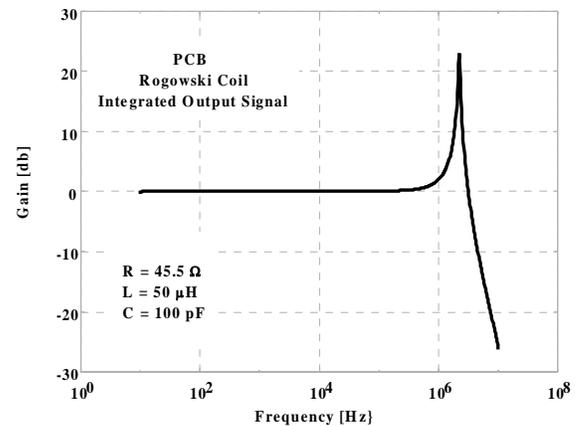
Figure 12. PCB Rogowski Coil Frequency response (integrated signal)
