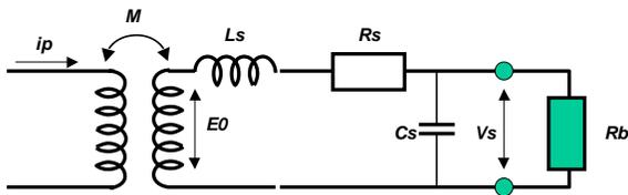
Figure 13a. Rogowski Coil Equivalent Circuit
