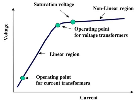
Figure 1. V-I Curve and Operating Points for Current and Voltage Transformers
