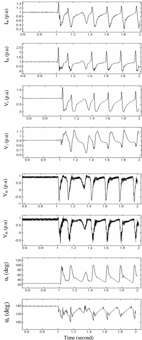
Fig. 5 System performance with conventional controllers during a 10% reduction of ESCR.
