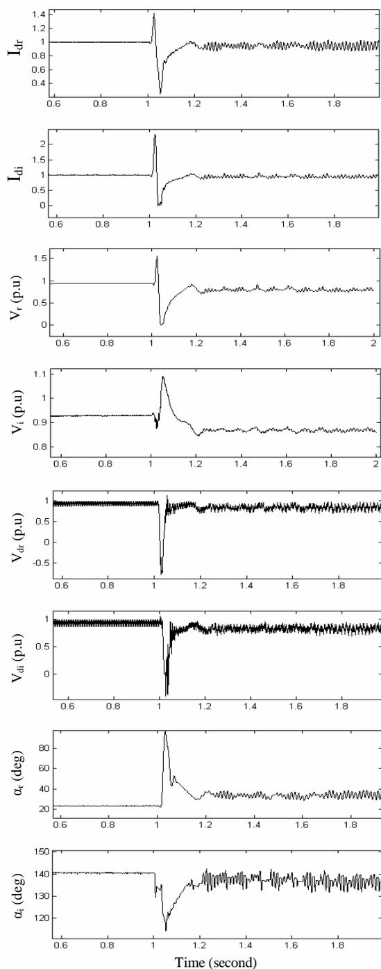
Fig. 6 System performance with proposed controller during a 10% reduction of ESCR.
