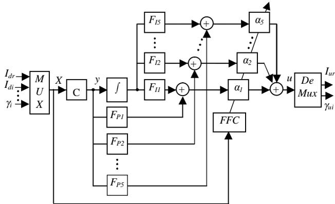
Fig. 4 Block diagram of proposed robust nonlinear fuzzy controller
