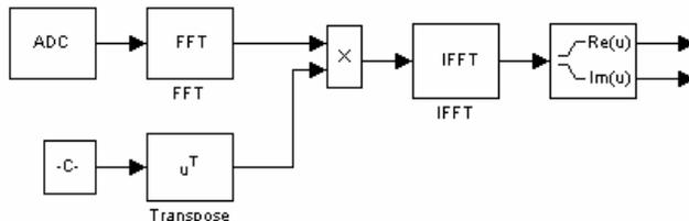
Fig. 1. Analytic Signal – Fast Fourier Transform approximation method
