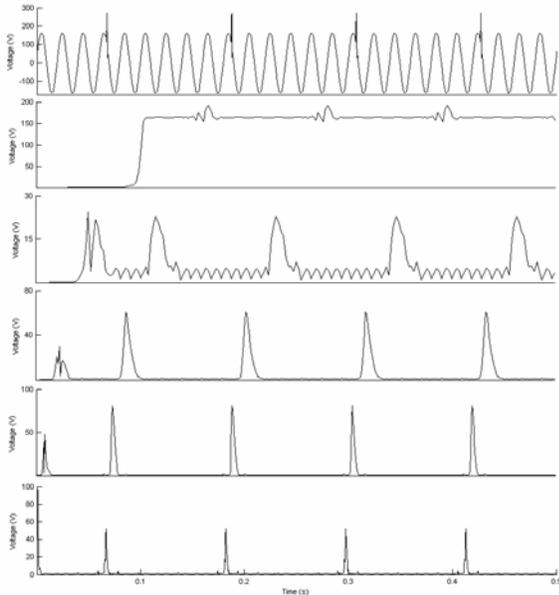
Fig. 7. Wavelet transform of analytic representation of measured voltage FFT approximation method. (a) Signal with a disturbance. DWT analysis (b) level 1 (lowest frequency). (c) level 2. (d) level 3. (e) level 4. (f) level 5 (highest frequency).
