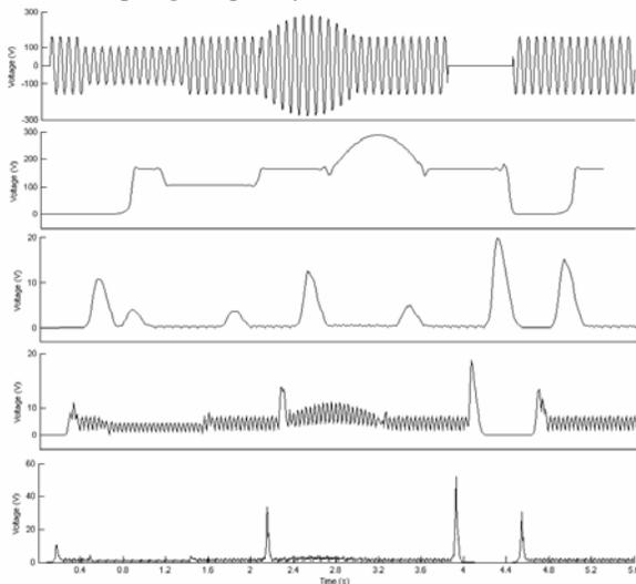
Fig. 11. Wavelet transform of analytic representation of measured voltage FIR approximation method for a signal with different PQ events.  $F_s=1.6\text{kHz}$ . DWT analysis (b) level 1 (lowest frequency). (c) level 2. (d) level 3. (e) level 4.(highest frequency).
