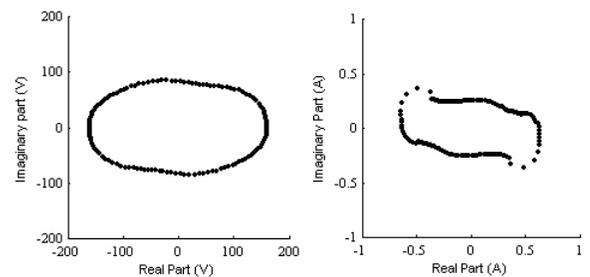
Fig. 5. Analytic representation of measured voltage and current FIR approximation method
