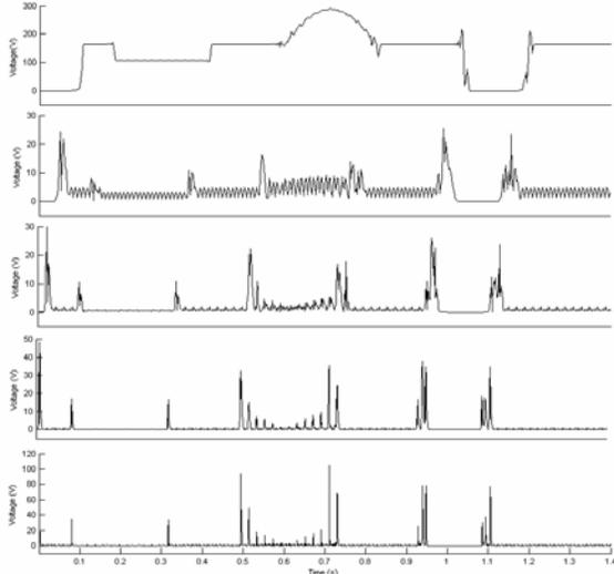
Fig. 10. Wavelet transform of analytic representation of measured voltage FFT approximation method for a signal with different PQ events. DWT analysis (a) level 1 (lowest frequency). (b) level 2. (c) level 3. (d) level 4. (e) level 5 (highest frequency).
