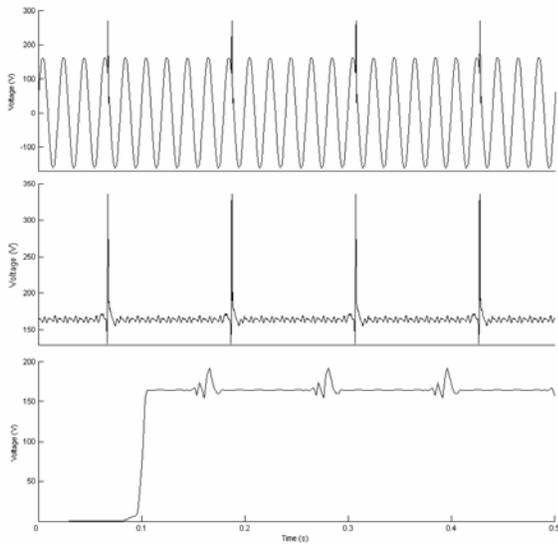
Fig. 6. Analytic representation of measured voltage FFT approximation method. (a) Signal with a disturbance. Envelope tracking using (b) AS-FFT. (c) Wavelet-AS-FFT (level 1).
