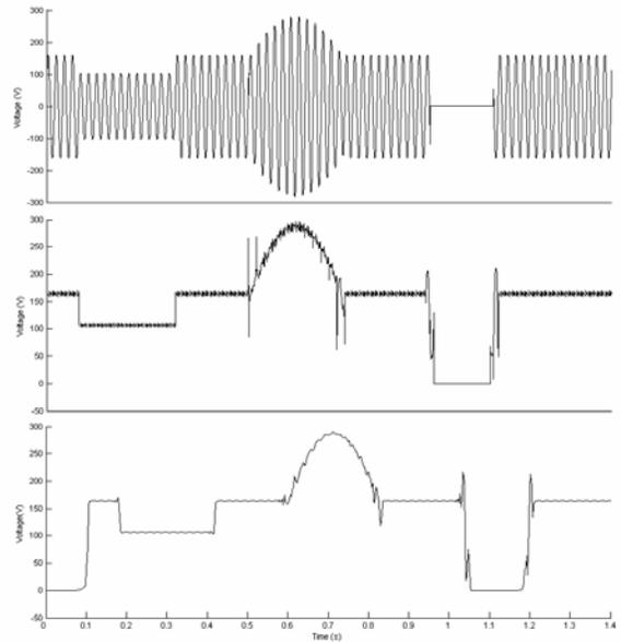
Fig. 9. Analytic representation of measured voltage FFT approximation method. (a) Signal with different PQ events. Envelope tracking using (b) AS-FFT. (c) Wavelet-AS-FFT (level 1-lowest frequency).
