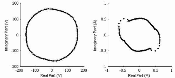
Fig. 4. Analytic representation of measured voltage and current FFT approximation method
