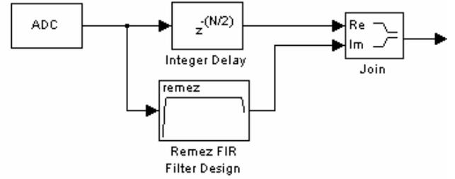
Fig. 2. Analytic Signal – Finite Impulse Response filter approximation method
