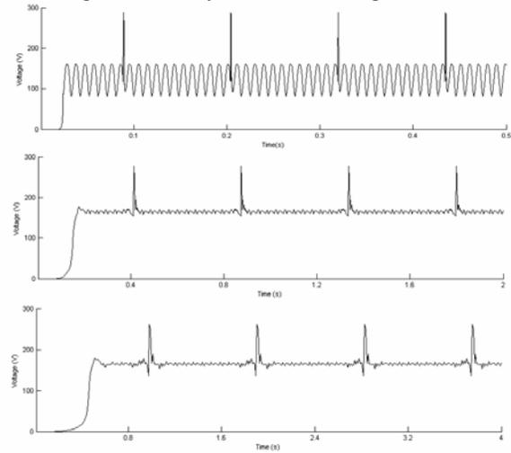
Fig. 8. Analytic representation of measured voltage FIR approximation method. Envelope tracking using (a) AS-FIR ( $F_s=6.4\text{kHz}$ ). (b) AS-FIR ( $F_s=1.6\text{kHz}$ ). (c) AS-FIR ( $F_s=800\text{Hz}$ )
