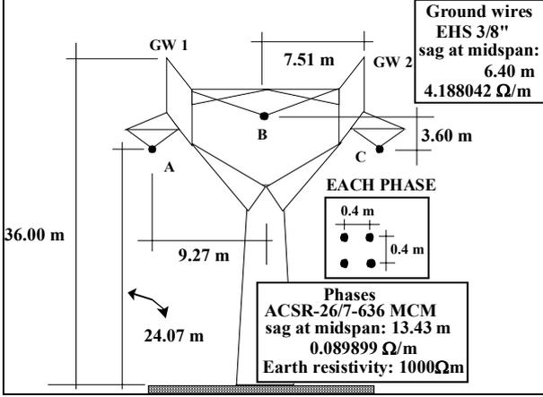
Fig. 3. Real three-phase line structure.
