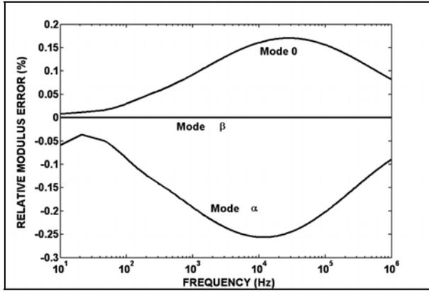
Fig. 4. Comparison between exact eigenvalues and quasi-mode results for symmetrical non-transposed three-phase line.
