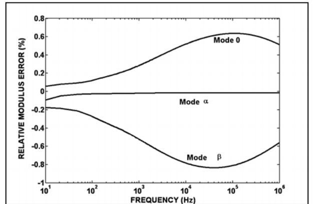
Fig. 6. Comparison between exact eigenvalues and quasi-mode results for design I (without vertical symmetry plane, non-transposed case).
