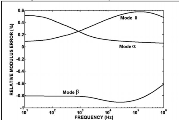
Fig. 7. Comparison between exact eigenvalues and quasi-mode results for design II (with the three phases centered in the same vertical plane, non transposed case).
