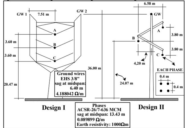
Fig. 5. Two designs for non-symmetrical three-phase line analyses.
