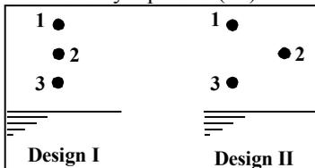
Fig. 5. Tree-phase line designs without vertical symmetry plane.
