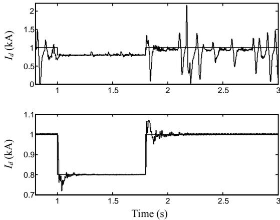
Fig. 4. Dynamic response of the system (top: pre-optimized parameter set; bottom: optimized parameter set)
