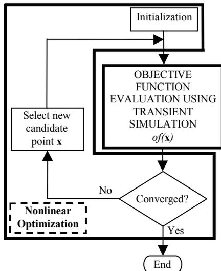
Fig. 1. Schematic diagram of the optimization-enabled transient simulation.
