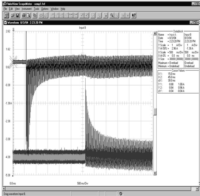
Fig.10 Phase-a currents of the transformers TR1 and TR2
