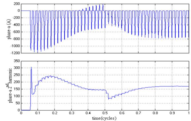
Fig.8 The transformer TR1 phase-a current and its 2<sup>nd</sup> harmonic component
