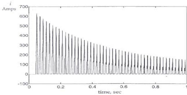
Fig.2 Typical inrush current
