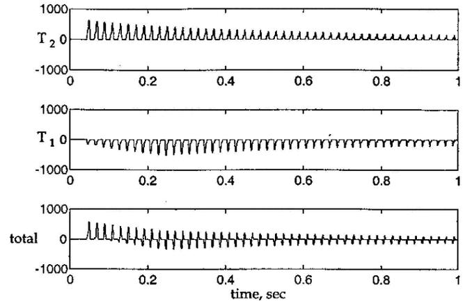
Fig.4 Typical sympathetic inrush currents
