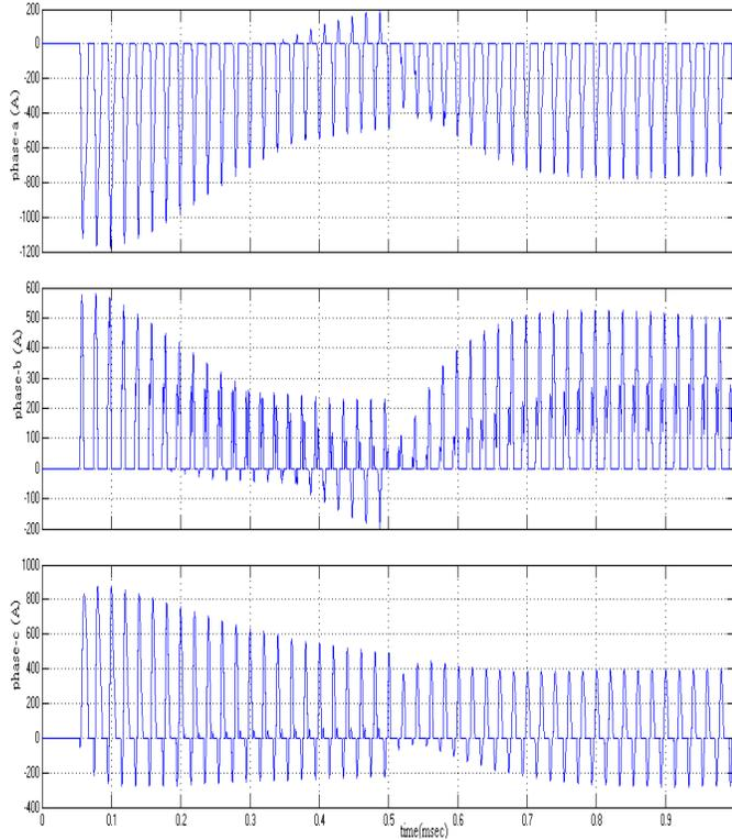
Fig.6 Phase currents of the transformer TR1
