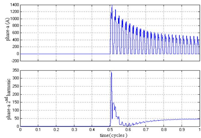
Fig.9 The transformer TR2 phase-a current and its 2<sup>nd</sup> harmonic component
