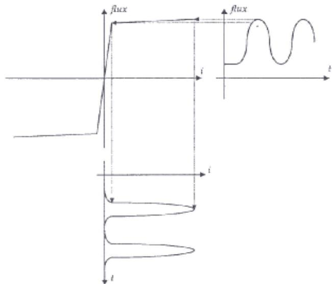
Fig.1 Illustration of the magnetizing inrush
