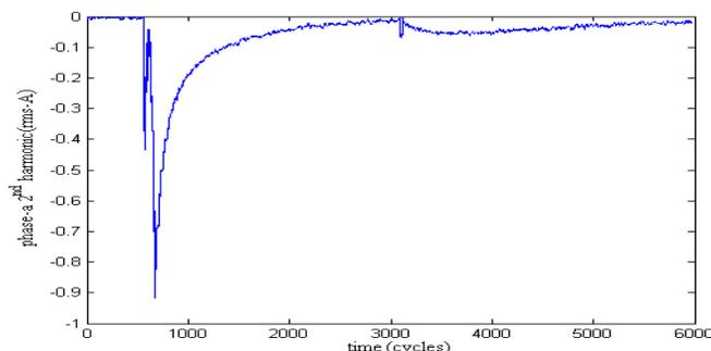
Fig.11 Phase-a current of the transformer TR1
