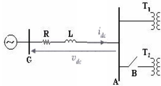
Fig.3 Connections leading to the sympathetic inrush
