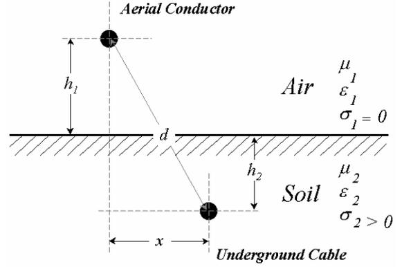
Fig. 1 Hybrid transmission system composed by an overhead aerial conductor and an underground power cable buried in an imperfectly conducting ground.
