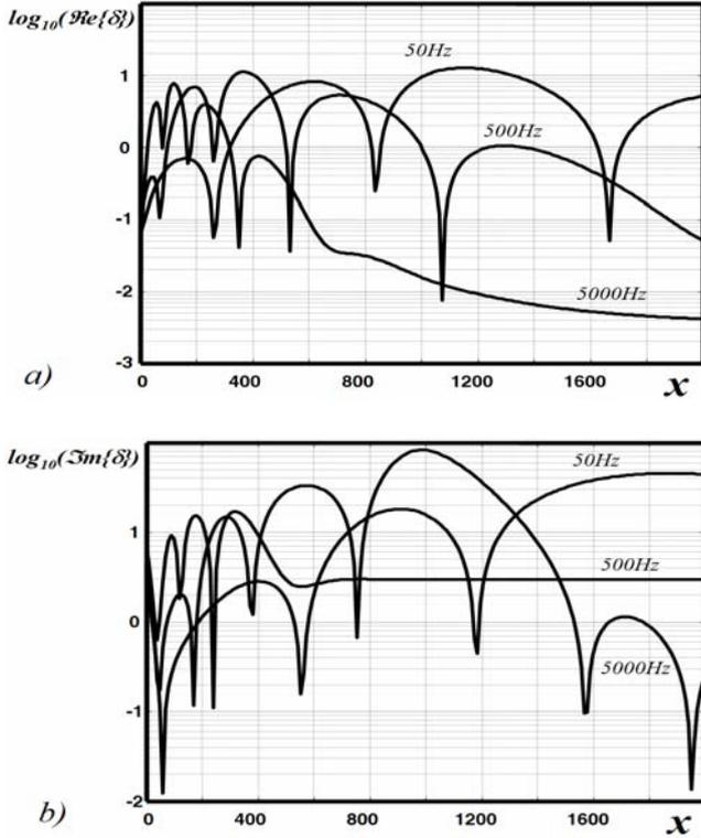
Fig. 5 Percent relative error level for the first application case between Pollaczek algorithmic solution and the formula proposed by Lucca [3]. a) Curves of  $\text{Re}\{\delta\}$ , b) Curves of  $\text{Im}\{\delta\}$ .
