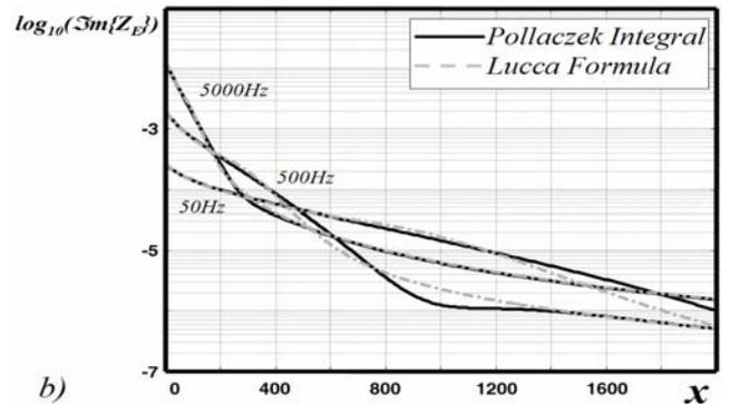
Fig. 4  $Z_E$  in dependency with the horizontal distance for the first application example [3]. a) Curves of  $\Re\{Z_E\}$ , b) Curves of  $\Im\{Z_E\}$ .
