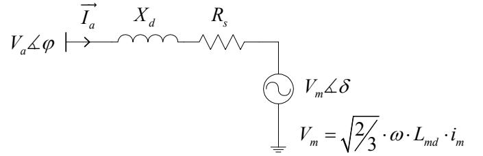
Fig. 8. Equivalent circuit of the machine in steady state
