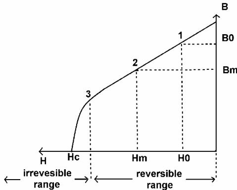
Fig. 3. Demagnetization curve of the permanent magnet [4]
