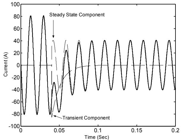
Fig. 9. Three phase short circuit current of the machines
