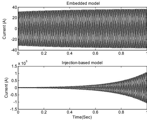
Fig. 10. Armature currents of the machines in time step  $167\mu\text{s}$
