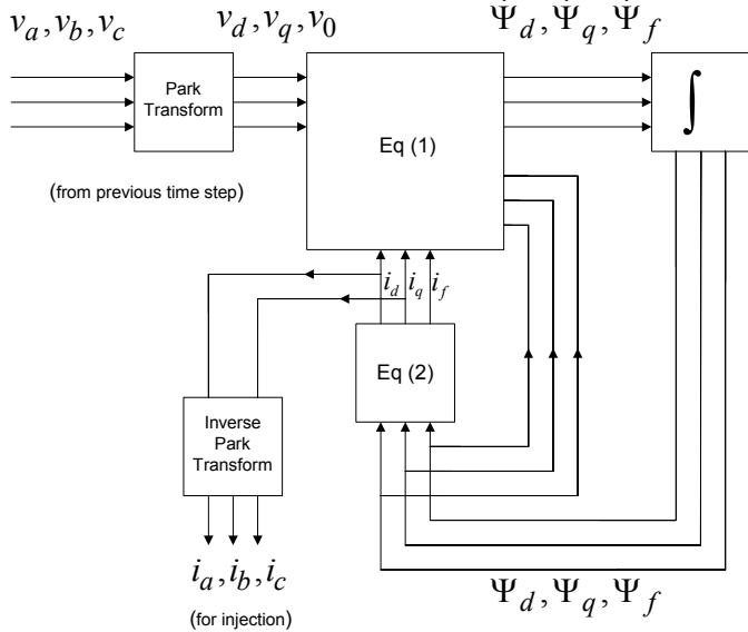
Fig. 5. Interfacing the machine to the network.
