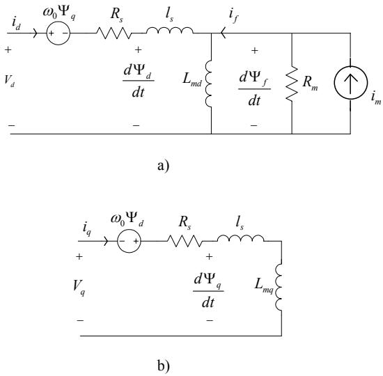
Fig. 2. Dq0 Equivalent circuit model of the PMSM a) D axis b) Q axis
