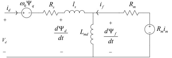
Fig. 4. D axis thevenin equivalent circuit of the PMSM
