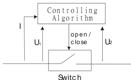
Fig. 1. Model of Vacuum circuit breakers
