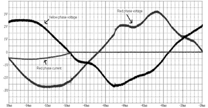
Fig. 5. Field test results – voltage at load side of the breaker
