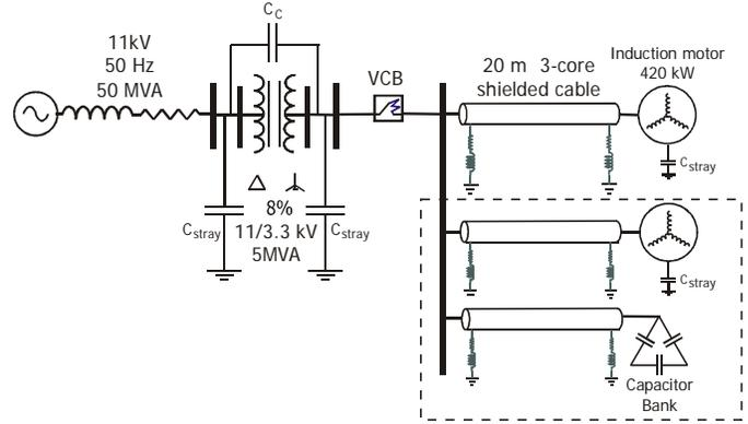
Fig. 3. Evaluation circuit to perform parametric sensitivity studies
