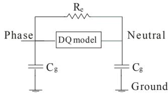
Fig. 2. Universal high-bandwidth hybrid model
