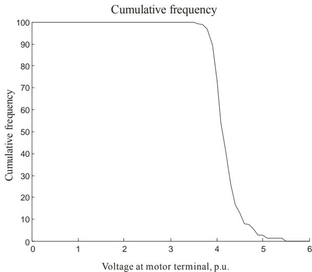
Fig. 7. Cumulative frequency of voltage at motor terminal without power factor correction capacitors
