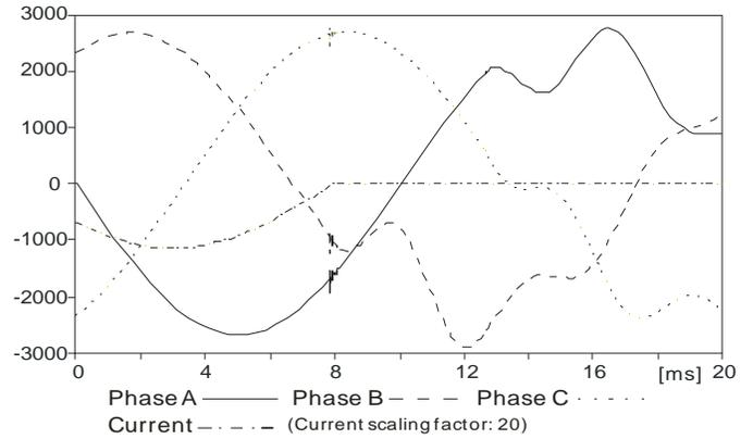
Fig. 6. Simulation results – voltage at load side of the breaker
