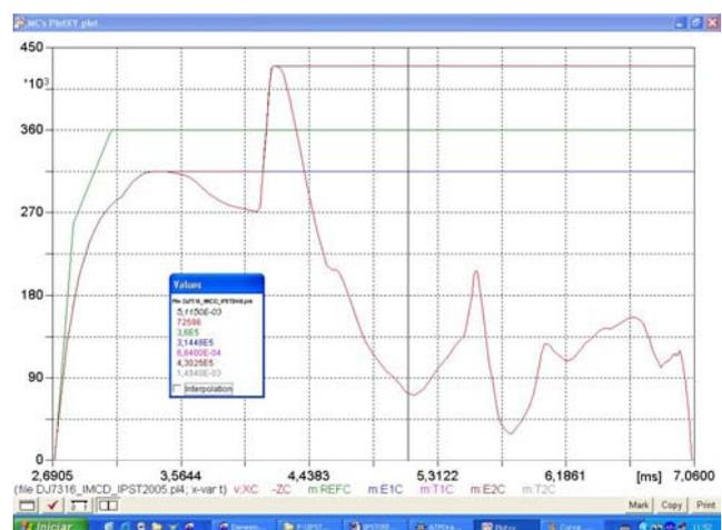
Fig. 6. TRV curve of the pole of phase C.
