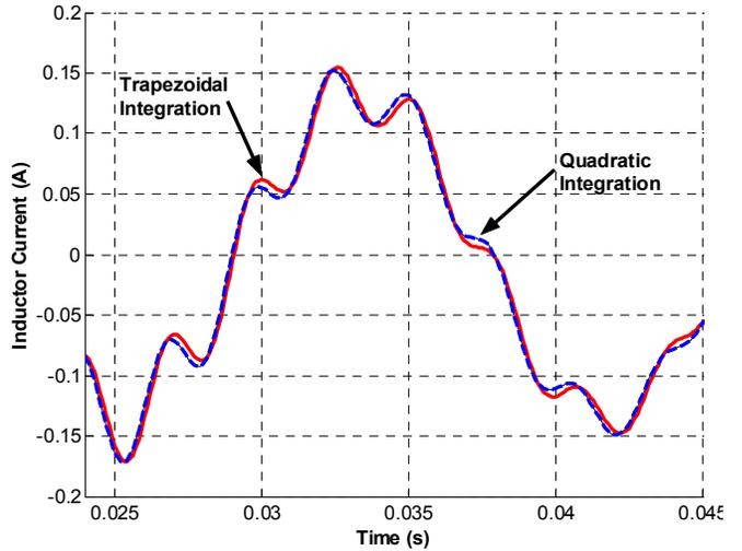
Fig. 4. Circuit current computed using trapezoidal (red) and quadratic (blue) integration.
