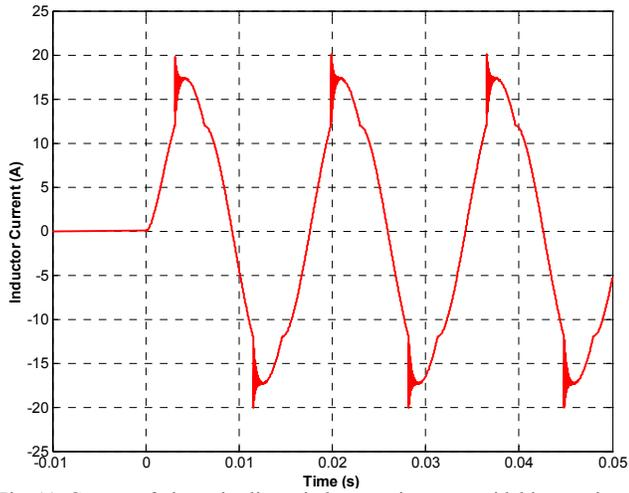
Fig. 11. Current of piecewise linear inductor using trapezoidal integration.
