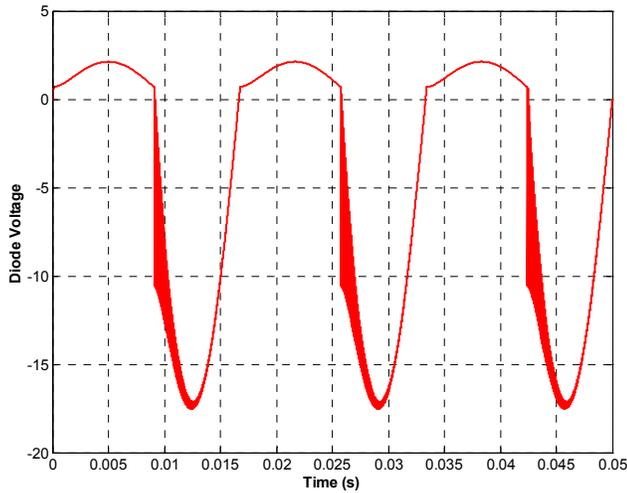
Fig. 16. Diode voltage using trapezoidal integration.
