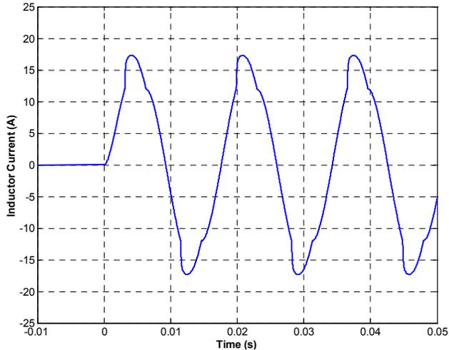
Fig. 13. Current of piecewise linear inductor using quadratic integration.
