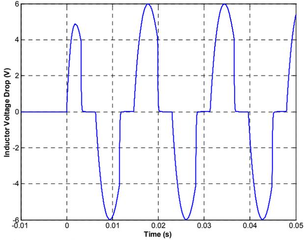
Fig. 12. Voltage of piecewise linear inductor using quadratic integration.
