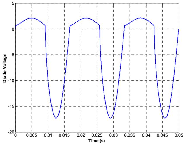
Fig. 18. Diode voltage using quadratic integration.
