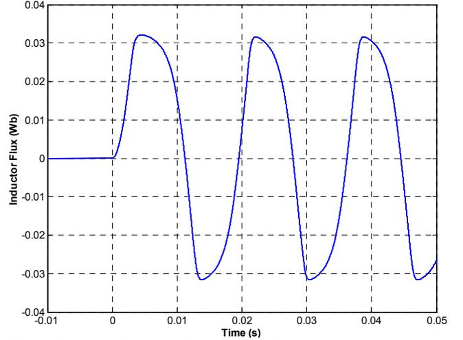
Fig. 9. Inductor flux waveform of a nonlinear inductor using quadratic integration.
