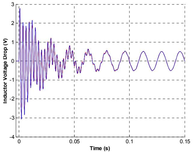
Fig. 5. Inductor voltage using trapezoidal (red) and quadratic (blue) integration.
