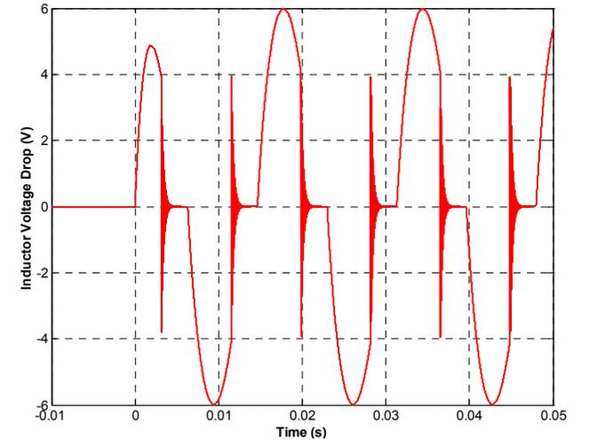
Fig. 10. Voltage of piecewise linear inductor using trapezoidal integration.
