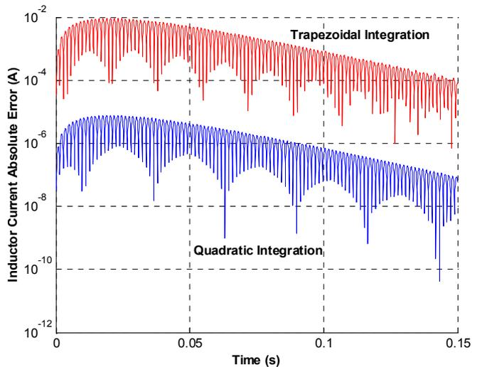
Fig. 6. Absolute error of circuit current of trapezoidal (red) and quadratic (blue) integration.
