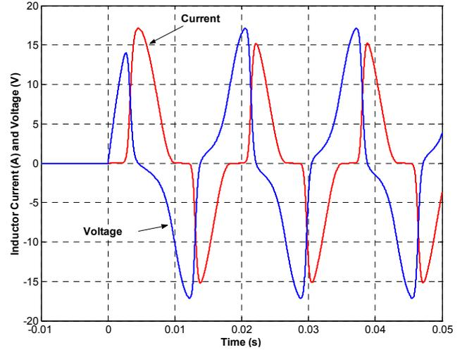
Fig. 8. Inductor voltage and current waveforms of a nonlinear inductor using quadratic integration.
