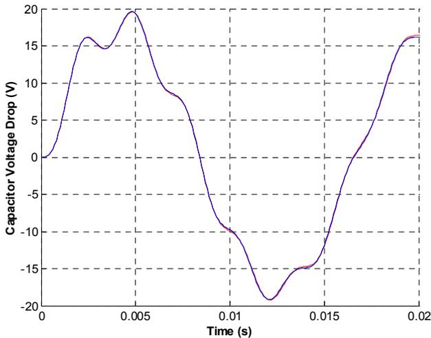
Fig. 3. Capacitor voltage computed using trapezoidal (red) and quadratic (blue) integration (waveforms are too close to be distinguished in the graph).
