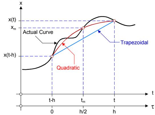
Fig. 1. Illustration of quadratic integration method.
