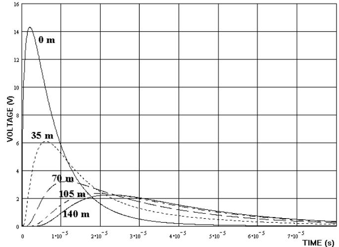
Fig. 5. Voltage distribution vs. time at various points of a 140 m long electrode buried in low relative permittivity soil ( $\epsilon_r=1$ ).
