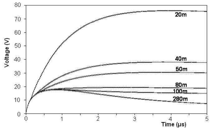
Fig. 6. Voltage distribution vs. time at injection (start) point of electrodes of various lengths ( $\epsilon_r=4$ ).
