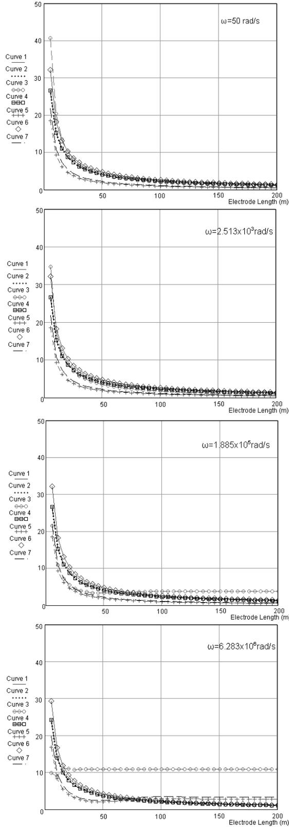
Fig. 1. Impedance magnitude of the grounding electrode as “seen” from one end, versus electrode length, when various calculation formulas are used.
