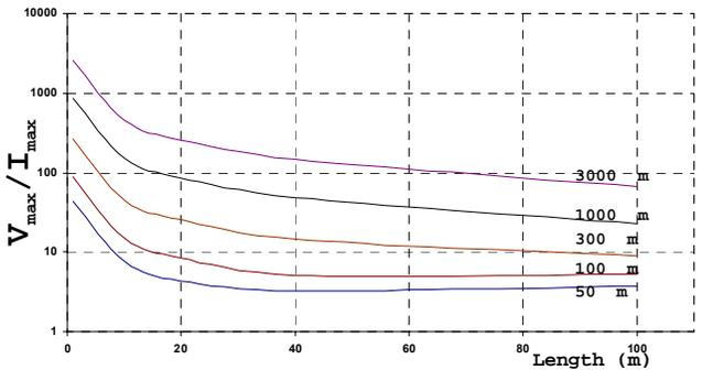
Fig. 8.  $V_{\max} / I_{\max}$  of horizontal conductors of various lengths under slow impulse.
