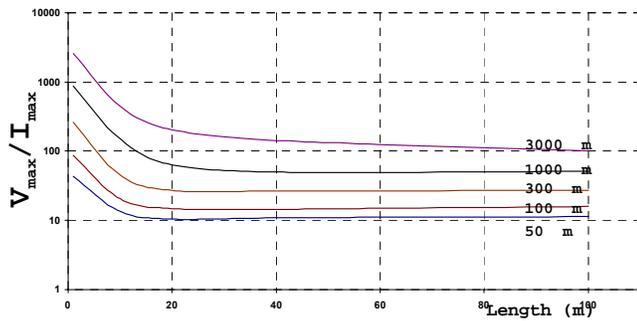
Fig. 7.  $V_{\max} / I_{\max}$  of horizontal conductors of various lengths under fast impulse.
