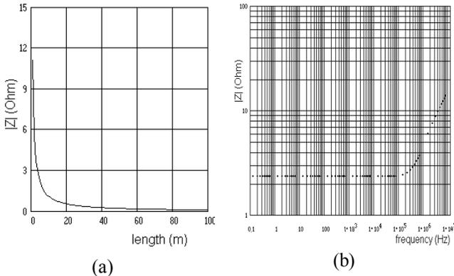
Fig. 4. Impedance magnitude of the grounding electrode as “seen” from one end, versus electrode length, when various calculation equations are used.
