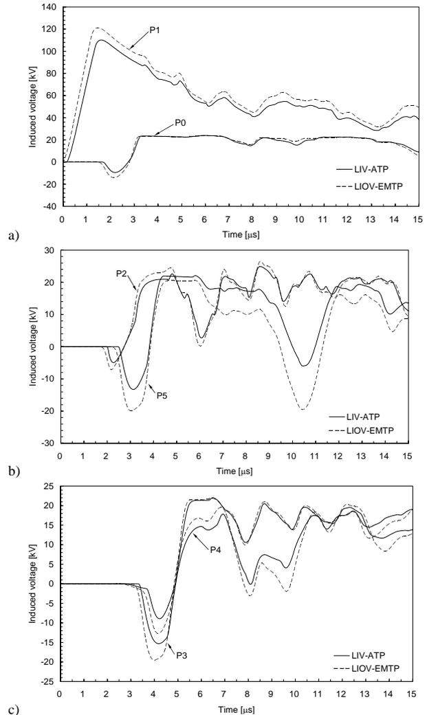
Fig. 9. Comparison between lightning-induced voltages on conductor #1 computed with LIV-ATP and LIOV-EMTP codes for the power distribution network of figure 7, stroke location #2; a) observation points P0 and P1; b) observation points P2 and P5; c) observation points P3 and P4.
