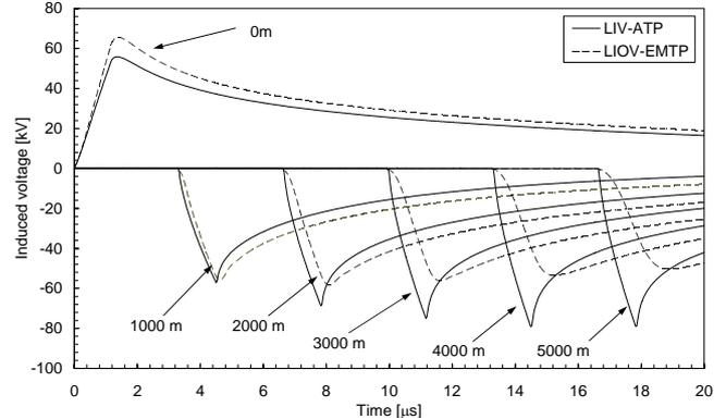
Fig. 6. Comparison between LIV-ATP and LIOV-EMTP codes for a 5 km overhead single conductor line; stroke location 50 m from left line termination, observation point placed each 1 km. Ground conductivity 0.001 S/m, relative permittivity 10. Stroke location # 3.
