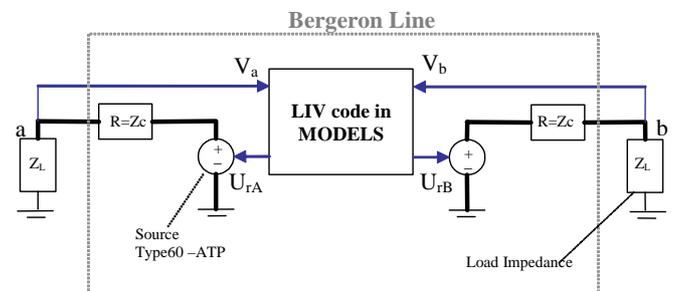
Fig. 2. Schematic representation of the interface of the LIV-ATP program for a single line. Adapted from [7].
