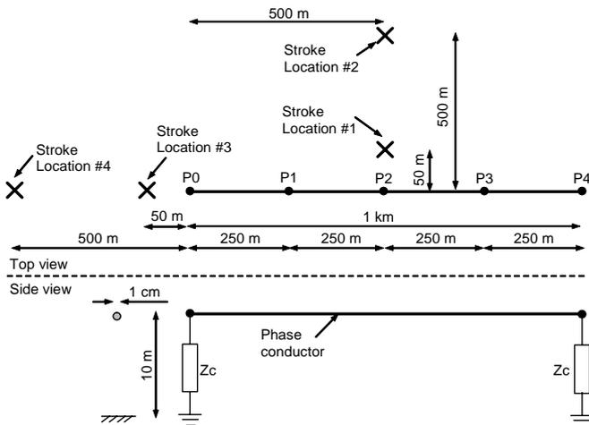
Fig. 3. Geometry adopted for the comparison between the LIOV-EMTP and LIV-ATP codes relevant to the single conductor straight line cases above ideal and lossy ground. The various stroke locations used for the simulations are shown in this figure.
