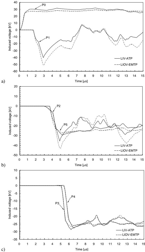
Fig. 8. Comparison between lightning-induced voltages on conductor #1 computed with LIV-ATP and LIOV-EMTP codes for the power distribution network of figure 7, stroke location #1; a) observation points P0 and P1; b) observation points P2 and P5; c) observation points P3 and P4.
