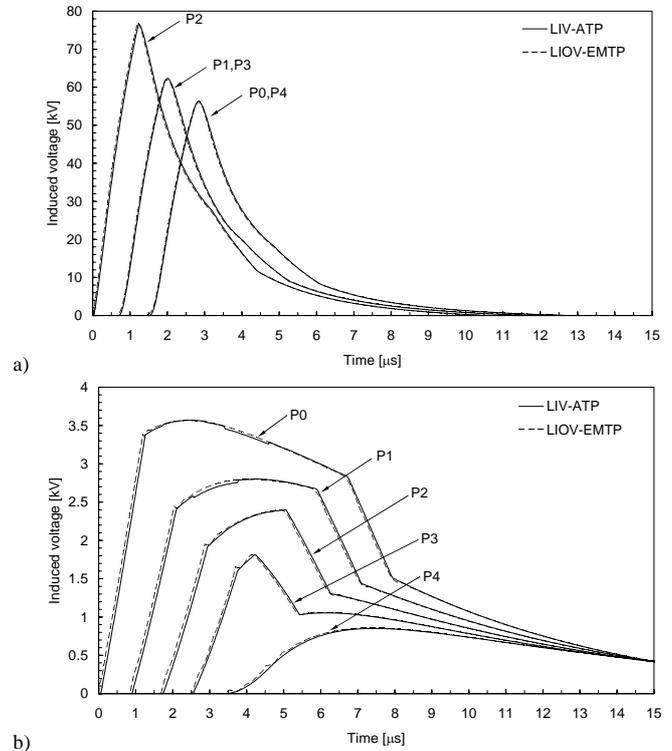
Fig. 4. Lightning induced voltages along the line (points P0 through P4 are defined in figure 3; a) stroke location #1, b) stroke location #4. The ground is assumed to be perfectly conducting.
