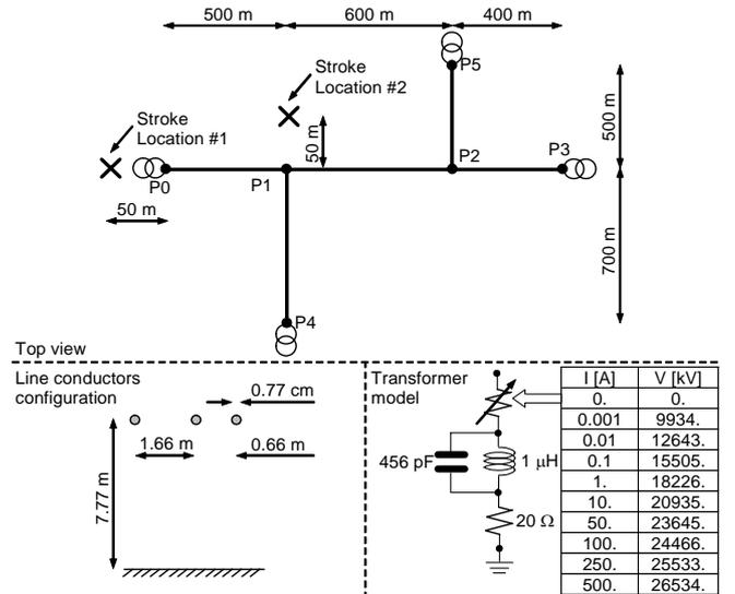
Fig. 7. Geometry adopted for the comparison between the LIOV-EMTP and LIV-ATP codes relevant to the complex distribution network case.
