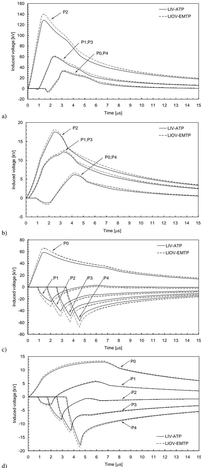
Fig. 5. Lightning induced voltages along the line (points P0 through P4 are defined in figure 3; a)stroke location #1, b)stroke location #2, c)stroke location #3, d)stroke location #4. Ground conductivity 0.001 S/m, relative permittivity 10.
