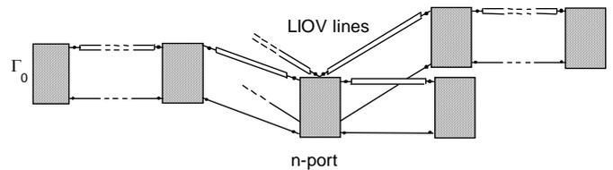
Fig. 1. Schematic representation of the electrical distribution system illuminated by LEMP in the LIOV-EMTP program. Adapted from [30].
