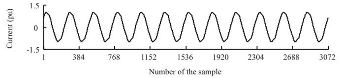
Fig. 13. Normalized current waveform of an actual oscillographic data without disturbance.
