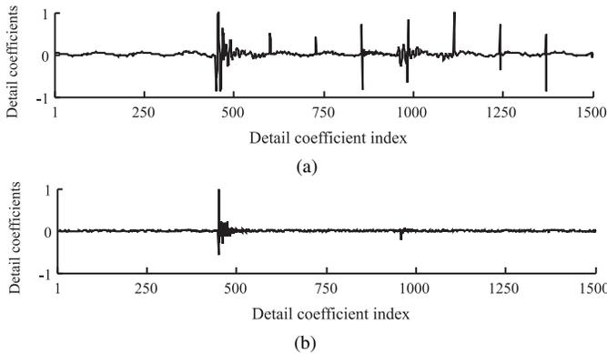
Fig. 12. Detail coefficients at scale 1 for phase A: (a) voltage; (b) current.
