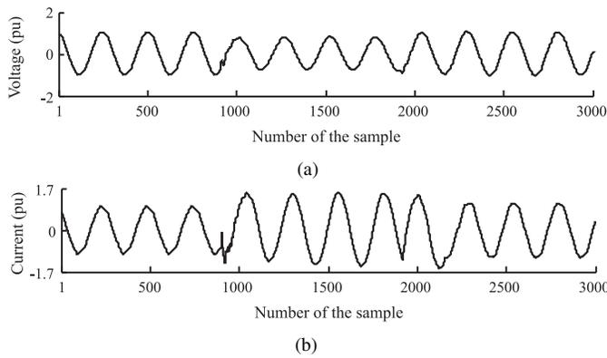
Fig. 11. Normalized waveforms of an actual voltage sag: (a) voltage; (b) current.
