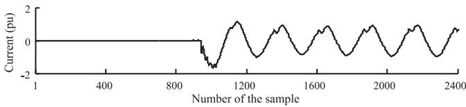
Fig. 5. Normalized current waveform of a transmission line energization transient.
