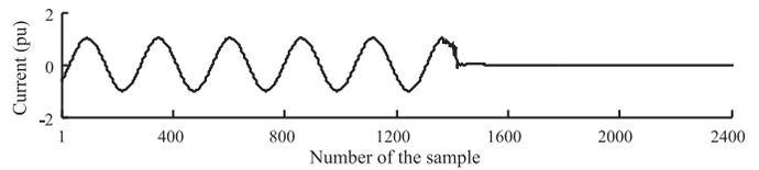
Fig. 7. Normalized current waveform of a transmission line de-energization transient.
