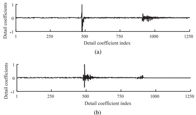
Fig. 10. Detail coefficients at scale 1: (a) voltage; (b) current.
