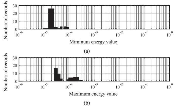
Fig. 17. Energy histogram for the oscillographic records without disturbance: (a) minimum values; (b) maximum values.
