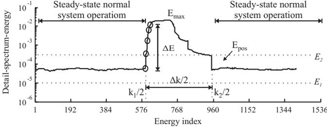
Fig. 16. Parameters at DSE curve for disturbance detection.
