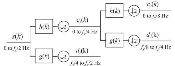
Fig. 1. DWT filter bank framework.
