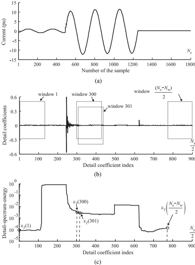
Fig. 2. Windowing: (a) original signal; (b) detail coefficients; (c) DSE
