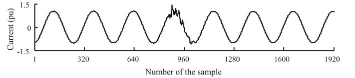
Fig. 3. Normalized current waveform of a capacitor energizing transient.
