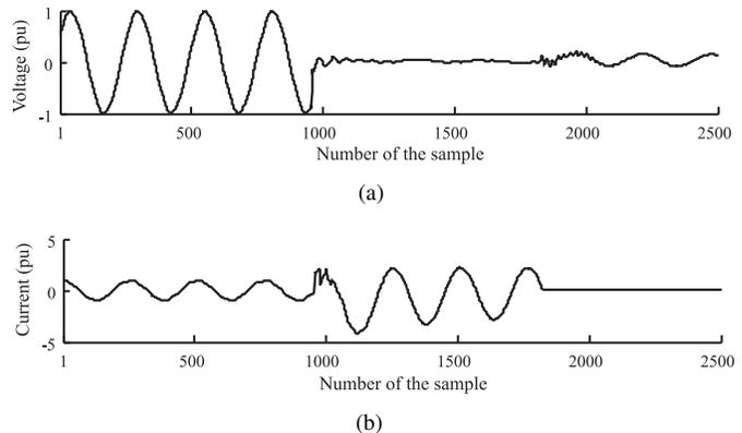
Fig. 9. Normalized waveform of an actual fault: (a) voltage; (b) current.
