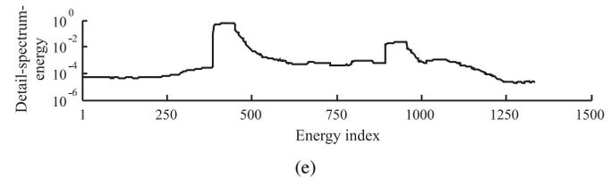
Fig. 15. DSE of the current, at scale 1, related to: (a) capacitor switching; (b) transmission line energization; (c) transmission line deenergization; (d) fault; (e) voltage sag.
