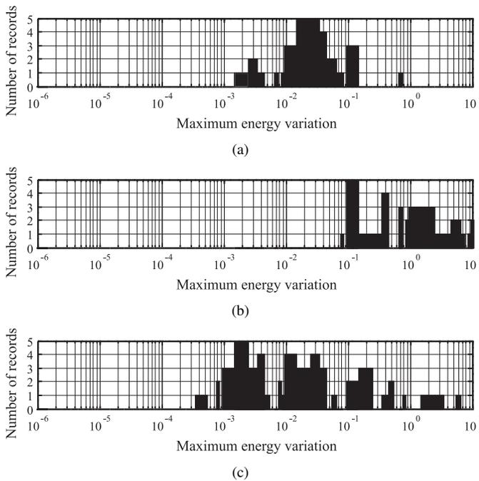
Fig. 18. Histogram of the maximum energy variation for the oscillographic records with: (a) transients due to capacitor switching; (b) fault; (c) sag.
