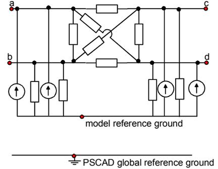
Fig. 2 Companion model with isolated model reference ground terminal.
