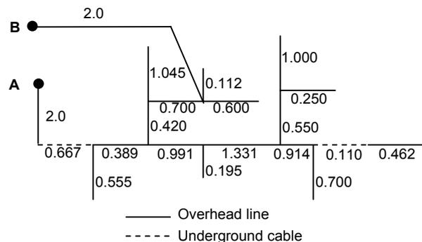
Fig. 6 Distribution system (lengths in km)
