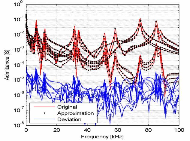
Fig. 8 Rational fitting of  $\mathbf{Y}$  ( $6 \times 6$ )
