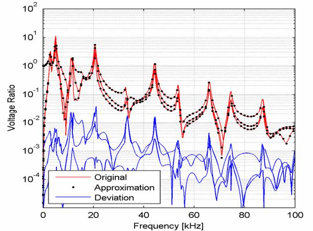
Fig. 10 Rational fitting of  $\mathbf{H}$  ( $1 \times 3$ )
