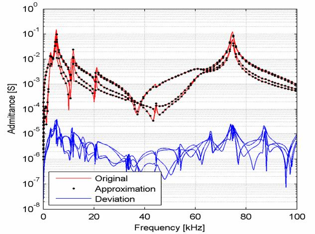
Fig. 9 Rational fitting of  $\mathbf{Y}^{red}$  ( $3 \times 3$ )
