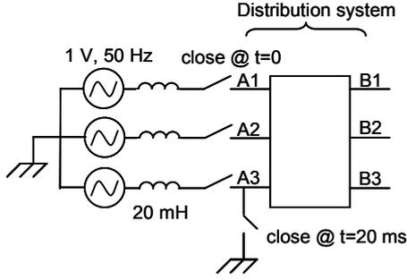
Fig. 7 Energization and ground fault initiation
