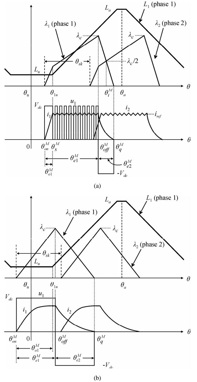
Fig. 2. Typical SRM waveforms in motoring operation considering the overlapping flux-linkage and current profiles of two neighboring phases: (a) PWM-current control and (b) single pulse control.
