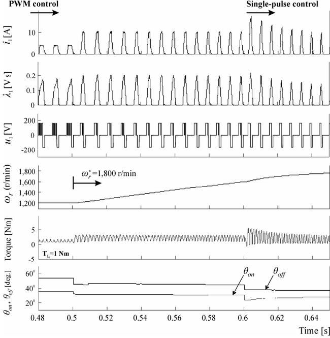
Fig. 6. Dynamic response of the optimal SRM drive to command speed step increase from 1,200 to 1,800 r/min, for load torque 1 Nm (current, flux-linkage and voltage of ph. 1, rotor speed, electromagnetic torque, turn-on and turn-off angles). The angles are counted from the aligned rotor position  $\theta_a$ .
