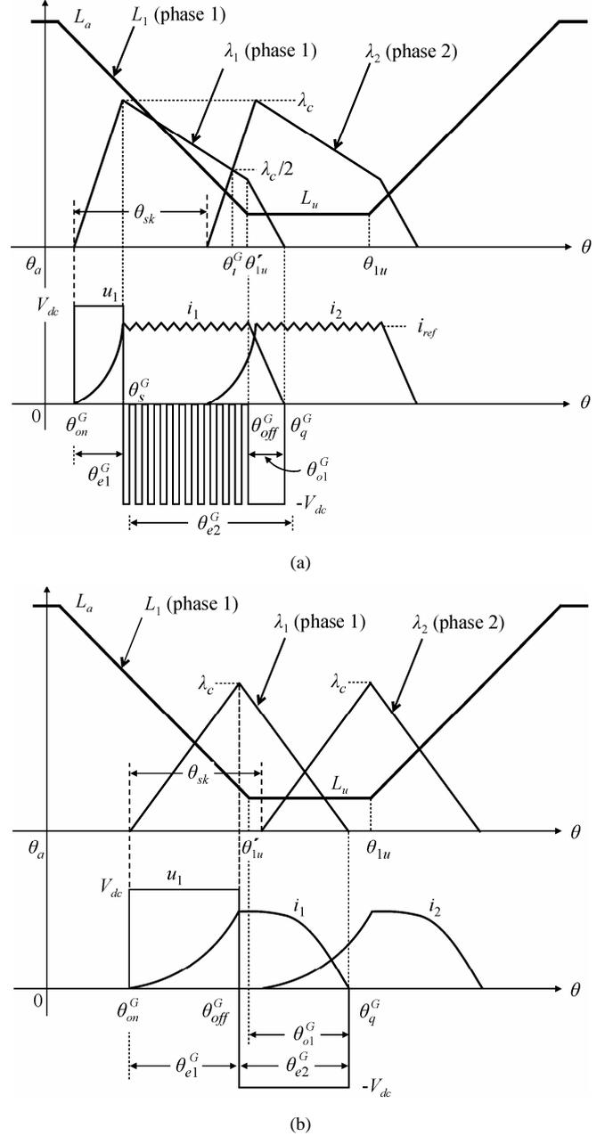
Fig. 3. Typical SRM waveforms in generating operation considering the overlapping flux-linkage and current profiles of two neighboring phases: (a) PWM-current control and (b) single pulse control.
