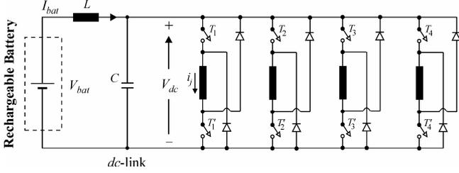
Fig. 1. Power converter topology of a 4-phase SRM.
