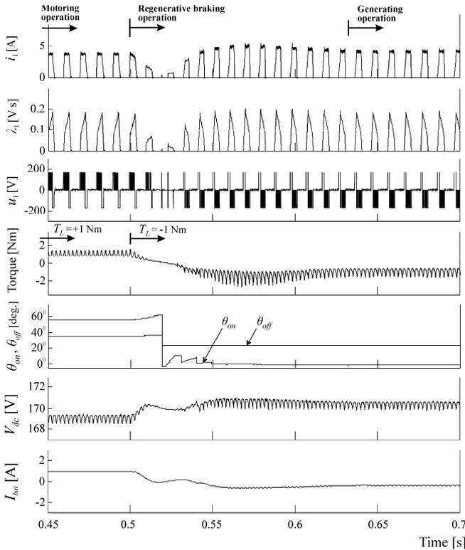
Fig. 8. Transient operation of the optimal SRM drive at 1,200 r/min with PWM control for a step change of applied torque from +1 Nm to -1 Nm (current, flux-linkage and voltage of ph. 1, electromagnetic torque, turn-on and turn-off angles, dc-link voltage and battery current). The angles are counted from the aligned rotor position  $\theta_a$ .
