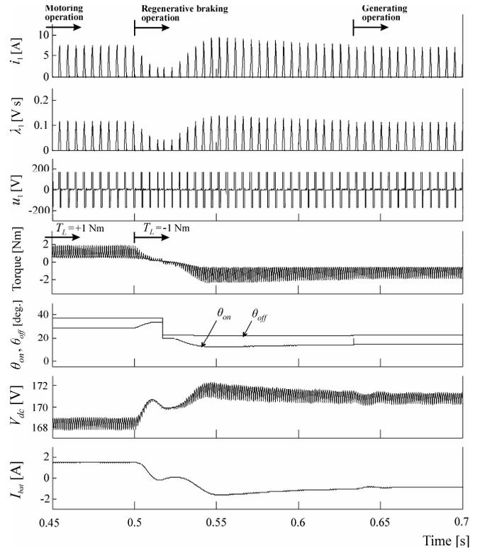
Fig. 9. Transient operation of the optimal SRM drive at 2,000 r/min with single pulse control for a step change of applied torque from +1 Nm to -1 Nm (current, flux-linkage and voltage of phase 1, electromagnetic torque, turn-on and turn-off angles, dc-link voltage and battery current). The angles are counted from the aligned rotor position  $\theta_a$ .
