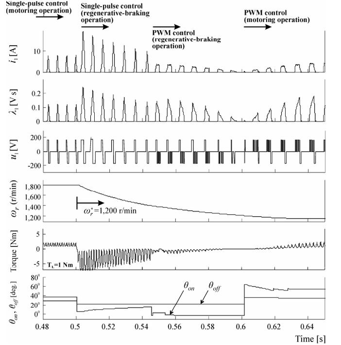
Fig. 7. Dynamic response of the optimal SRM drive to command speed step decrease from 1,800 r/min to 1,200 r/min, for load torque 1 Nm (current, flux-linkage and voltage of ph. 1, rotor speed, electromagnetic torque, and turn-on and turn-off angles). The angles are counted from the aligned rotor position  $\theta_a$ .
