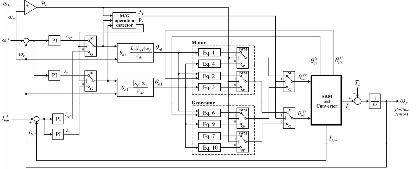
Fig. 4 Block diagram of a universal SRM control system for optimal motoring and generating operation.
