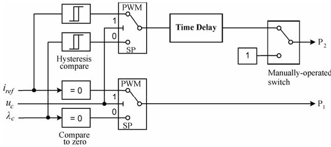
Fig. 5. M/G operation detector control scheme.
