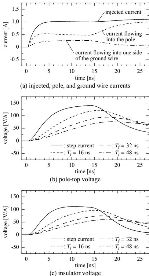
Fig. 11. Calculated results using the proposed EMTP model in Case 3.
