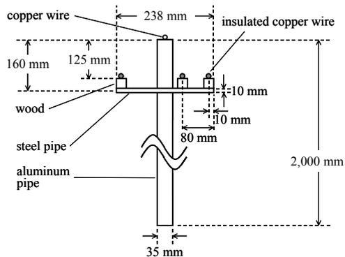
Fig. 1. Reduced-scale distribution line model.
