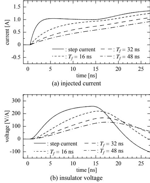
Fig. 10. Calculated results using the proposed EMTP model in Case 2.
