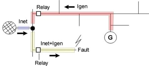
Fig. 1. Sympathetic tripping in distribution network.
