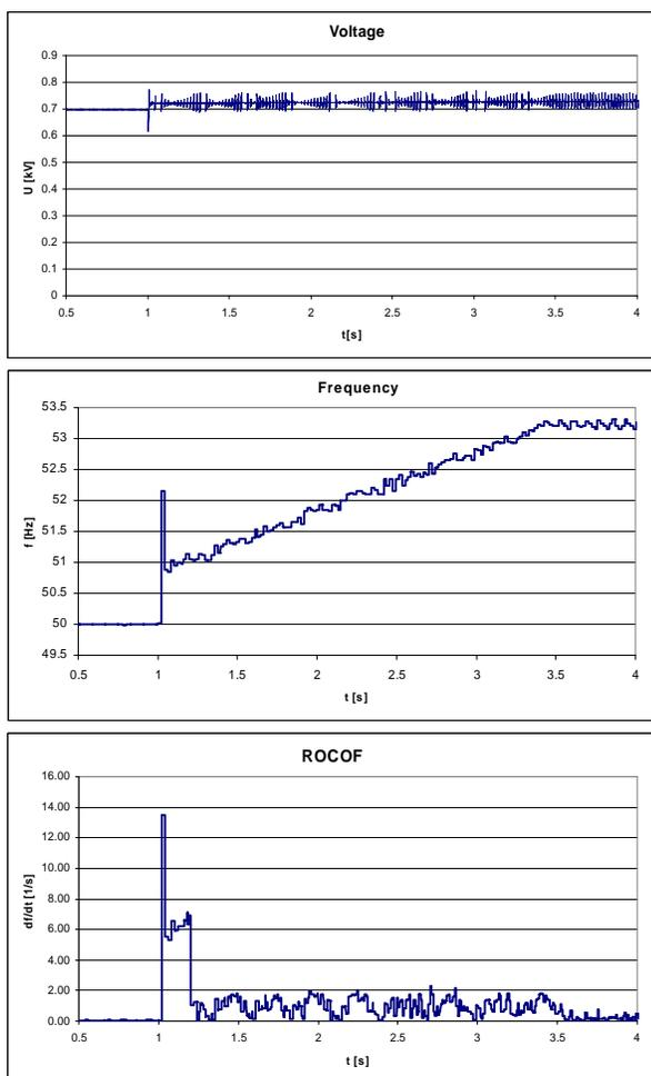
Fig. 10. Islanding detection measurements.
