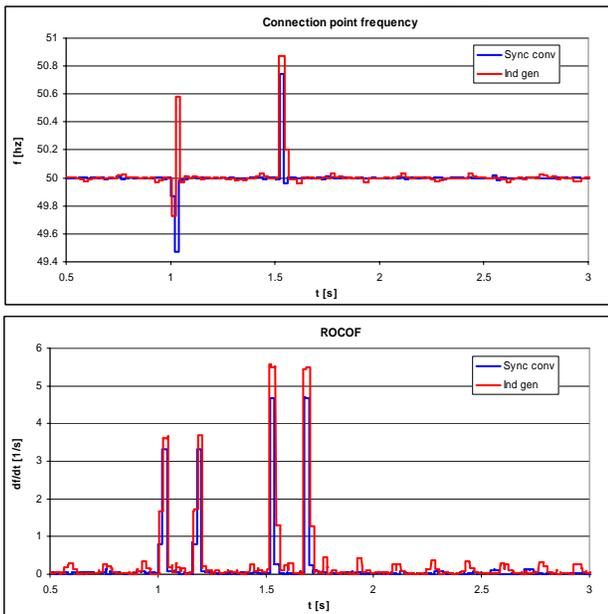
Fig. 9. Frequency and ROCOF measurements.
