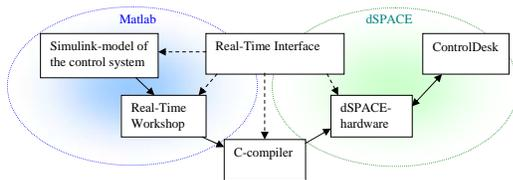
Fig. 4. The connections between dSPACE and Matlab.
