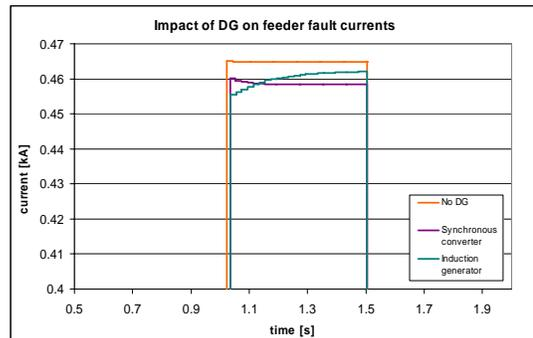
Fig. 6. The blinding effect remains minor.
