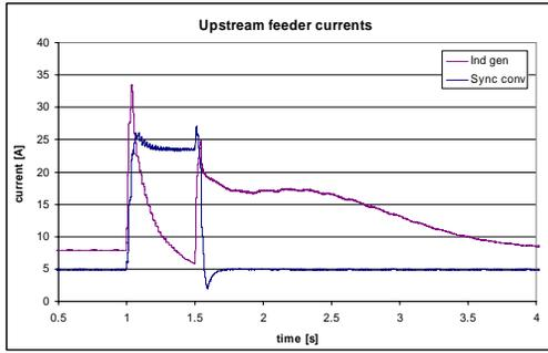
Fig 7. Upstream currents during a short circuit located at the substation bus. Fault occurs at 1 s and becomes cleared after 0.5 s.
