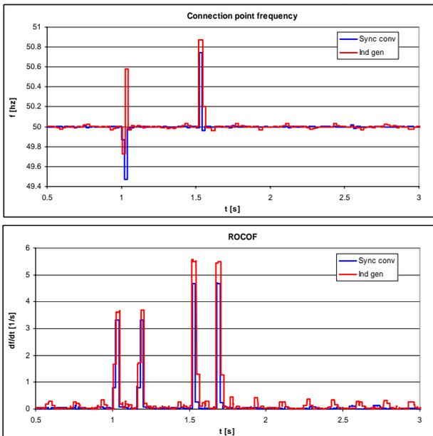
Fig. 9. Frequency and ROCOF measurements.
