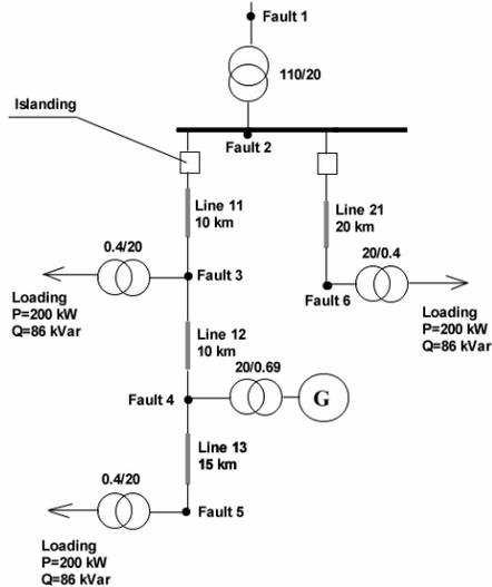
Fig. 5. The example case used in the simulations.
