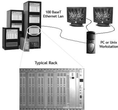
Fig. 3. Typical RTDS configuration. [11]
