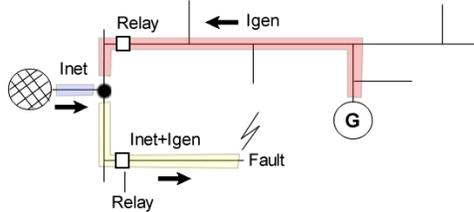
Fig. 1. Sympathetic tripping in distribution network.
