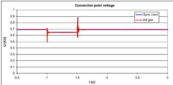
Fig. 8. Voltage drop at the DG connection point during fault in point 6.
