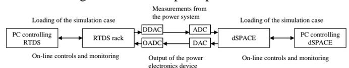
Fig. 2. The connection of RTDS and dSPACE simulators.
