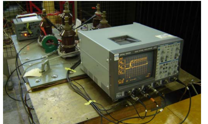
Fig. 6. Recording equipment for measurements of fast transient oscillations.
