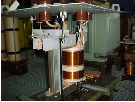
Fig. 1. Test transformer during production in the factory.
