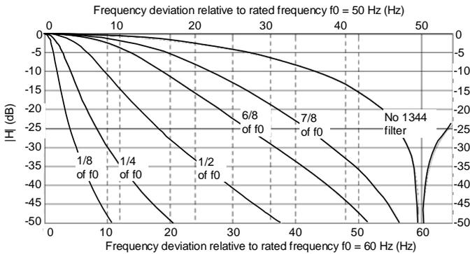
Fig. 1. Attenuation of PMU on subsynchronous frequency range [6]
