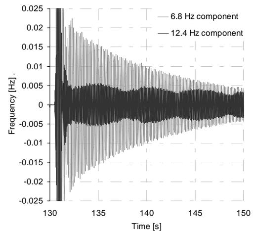
Fig 6. Frequency components for 6.8 Hz and 12.4 Hz torsional mode obtained from measured frequency using narrow band pass filters
