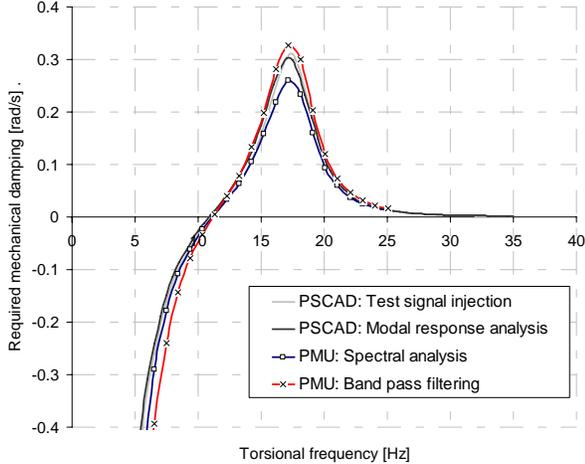
Fig 11. Comparison of PMU based results with simulation results obtained using PSCAD for System-1 with 75 % degree of series compensation
