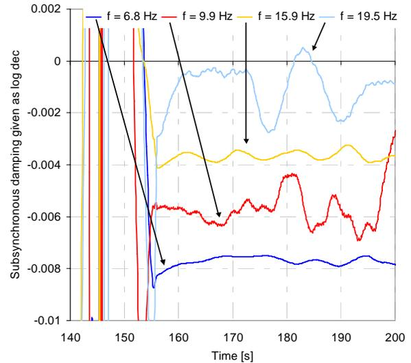
Fig 13. Subsynchronous damping calculated using results of spectral analysis performed for rate of change of frequency
