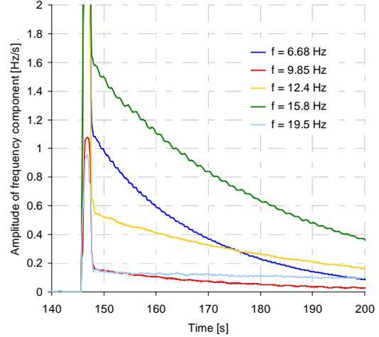
Fig 12. Attenuation of torsional components determined using standard deviation of the band-pass filtered rate-of-change of frequency
