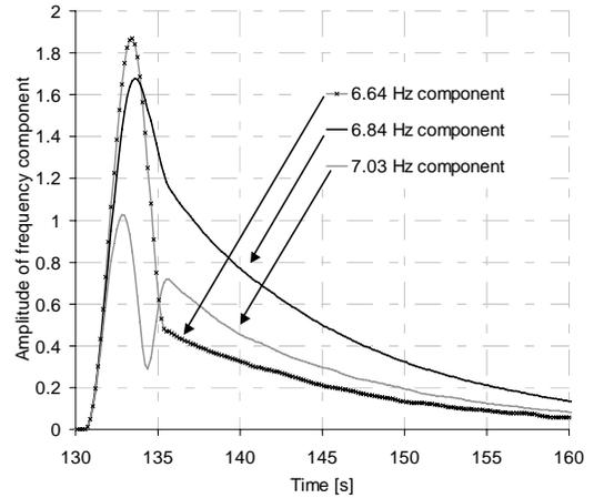
Fig 5. Shape of the subsynchronous frequency components
