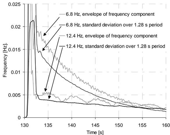
Fig 7. Envelope curve and standard deviation of 6.8 Hz and 12.4 Hz frequency component
