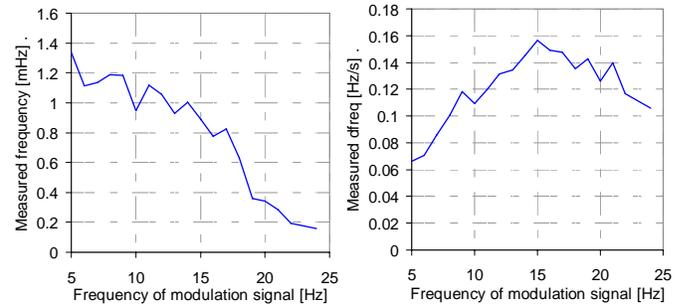
Fig 9. Frequency response of PMU for small amplitude (2.5 mHz) modulation of generator speed on subsynchronous frequency range
