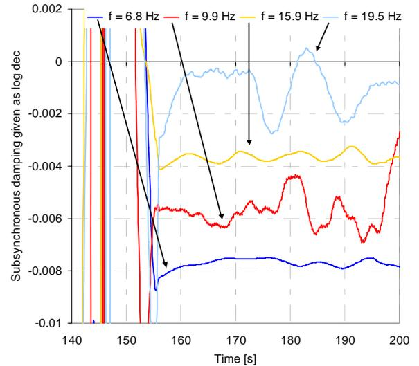
Fig 13. Subsynchronous damping calculated using results of spectral analysis performed for rate of change of frequency
