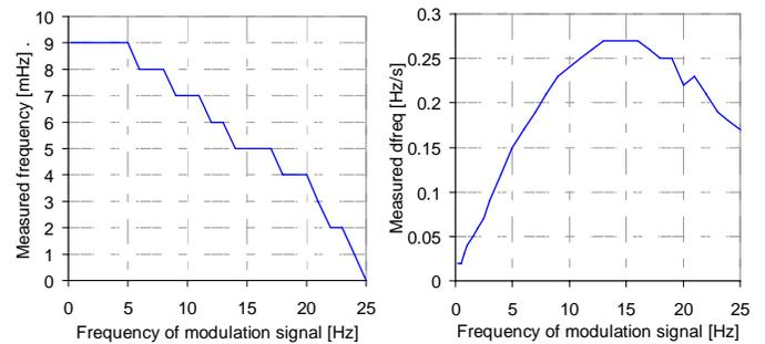
Fig 8. Inherent attenuation of PMU for frequency modulation using peak-to-peak amplitude of 10 mHz on subsynchronous frequency range
