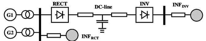
Fig. 3. Structure of the AC-DC-system model used in tests
