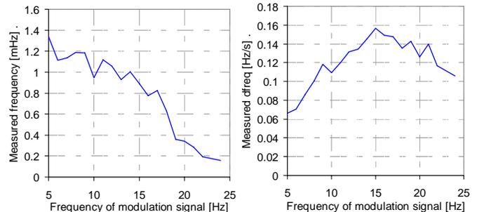
Fig 9. Frequency response of PMU for small amplitude (2.5 mHz) modulation of generator speed on subsynchronous frequency range
