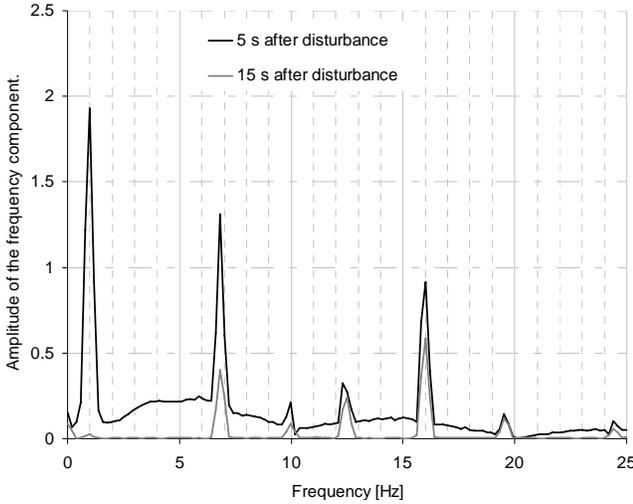
Fig. 4. Post-disturbance frequency spectrum determined based on PMU frequency measurement signal
