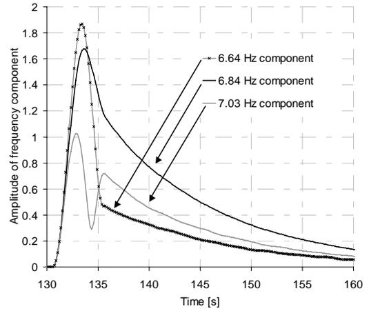
Fig 5. Shape of the subsynchronous frequency components
