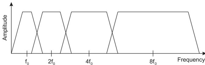
Fig. 1. Frequency spectrum using the Discrete Wavelet Transform.
