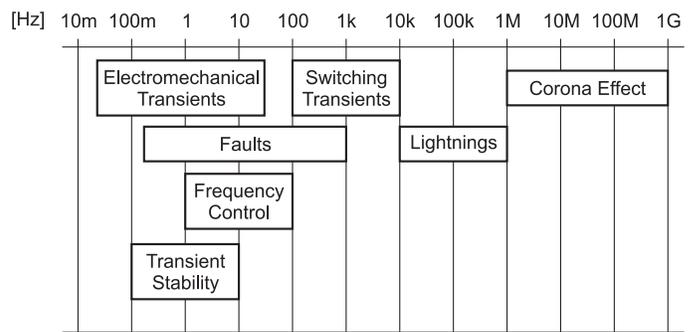
Fig. 2. Frequency spectrum of power system transients.
