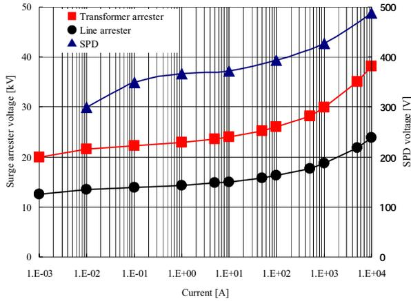
Fig. 6. Voltage-current characteristics of surge arresters and SPD
