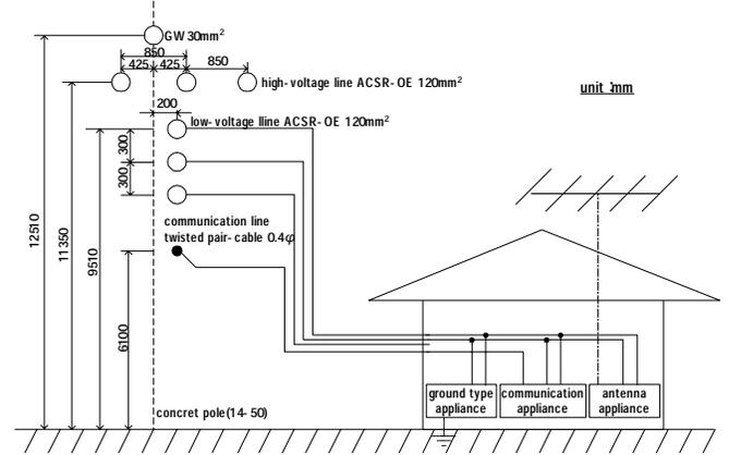
Fig. 3. Configuration of distribution and communication lines
