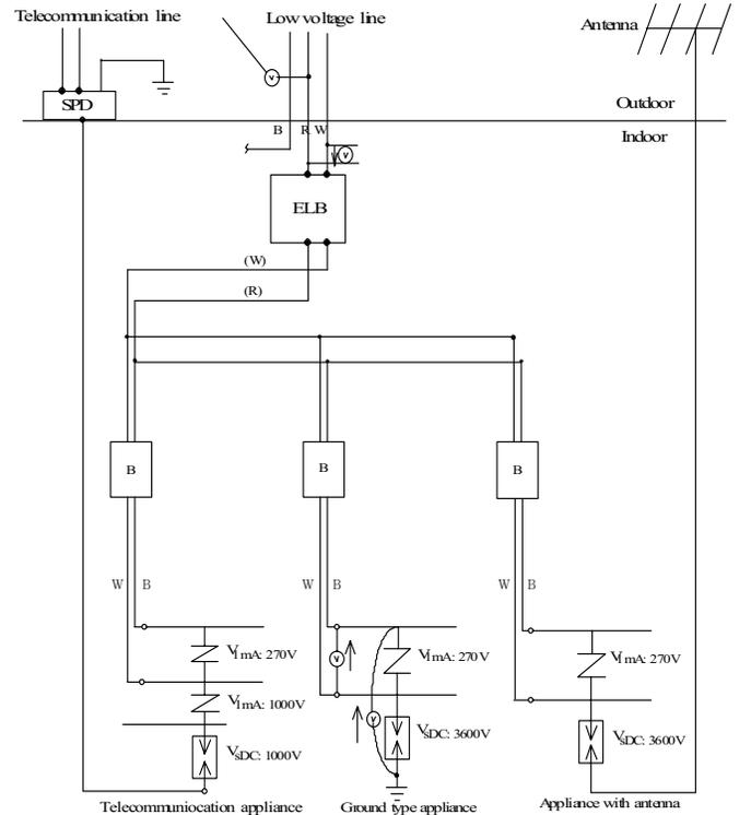
Fig. 4. Low voltage circuit in a residence
