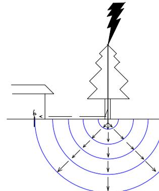
Fig. 1. A simplified model of lightning hit to ground associated with voltages in residence.
