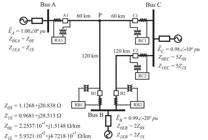
Fig. 1. Diagram of the test power system.
