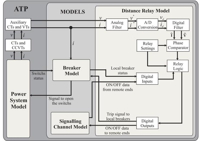
Fig. 2. Overall block diagram of the simulation using MODELS.
