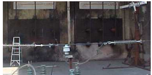
Fig. 2. Layout for experiment involving a pierced clad conductor.
