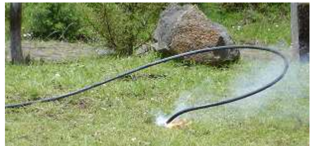
Fig. 8. 13.8 kV conductor laid on wet grass.
