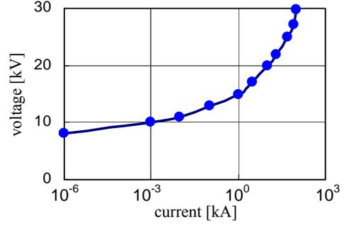
Fig.5. Linear-wise characteristics model for 2.5-kA surge arrester.
