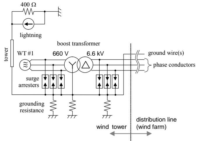
Fig. 2 Detail model of each wind turbine
