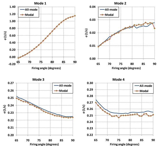
Fig. 6. Damping of modes 1-4 with all-mode and modal models when TCSC is utilized
