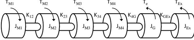
Fig. 1. General representation of six-mass shaft system
