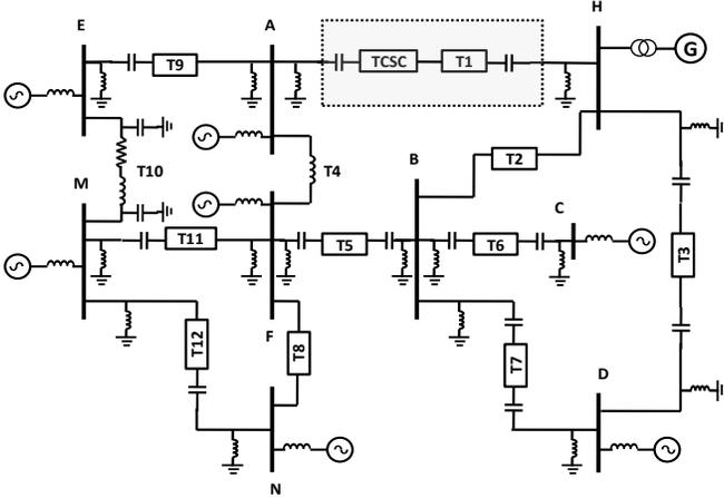
Fig. 3. Single line representation of studied power system
