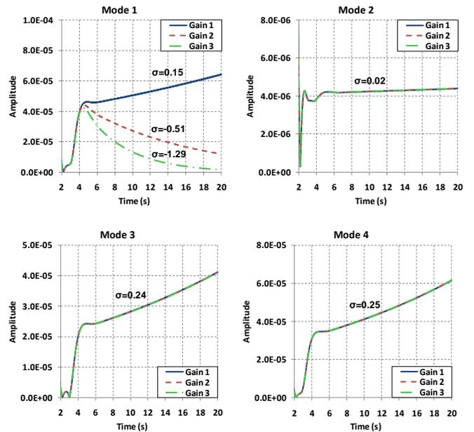
Fig. 8. Effect of gain of mode 1 SSDC on oscillation amplitudes
