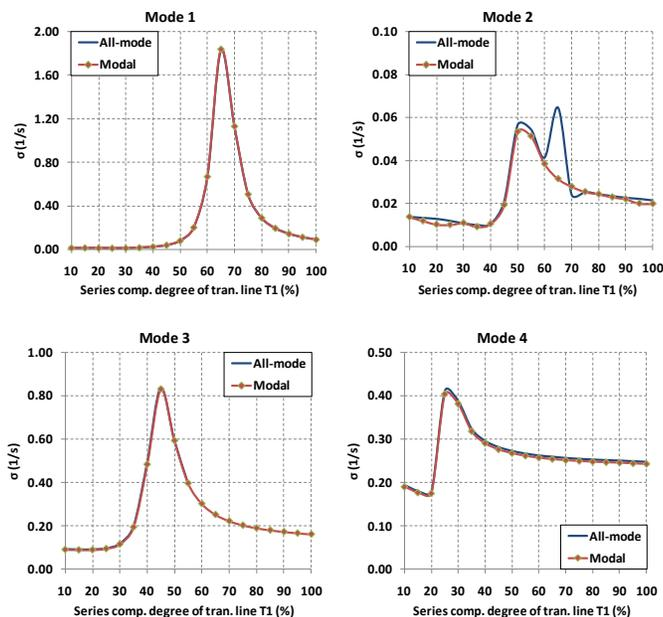
Fig. 5. Damping of modes 1-4 with all-mode and modal models
