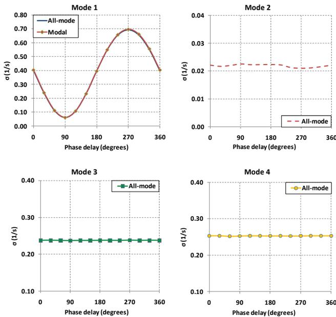
Fig. 7. Effect of phase shift of mode 1 SSDC on oscillations damping with all-mode model
