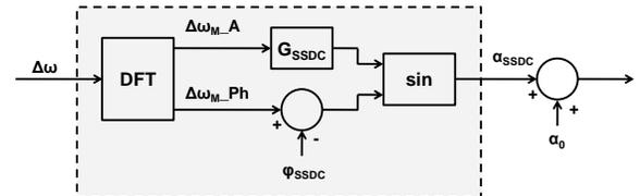
Fig. 4. Structure of the generic SSDC circuit applied in the study
