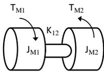
Fig. 2. Two-mass model for modal modeling of turbine-generator shaft
