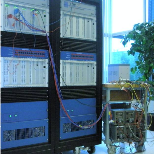
Fig. 7. Closed-loop relay test circuit.
