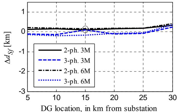
Fig. 11.  $\Delta d_{sf}$  with compensation B. All faults are at the end of the feeder, while the connection point of the DG is varied. Low load.
