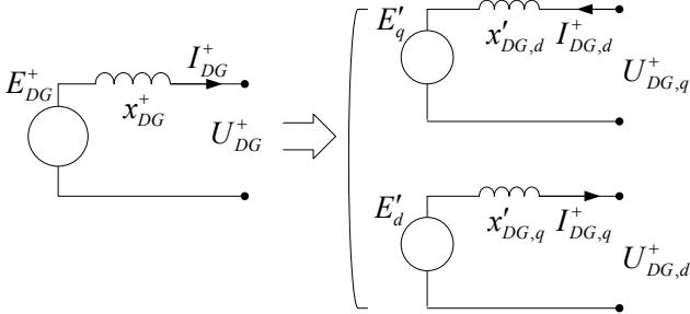
Fig. 7. Positive sequence equivalent circuit for the transient state
