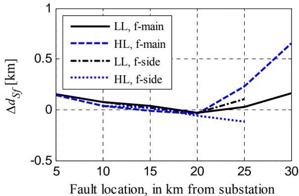
Fig. 13.  $\Delta d_{sf}$  with compensation B for feeder with three DG-units. All faults are 2-phase short-circuits, and the fault location is varied.
