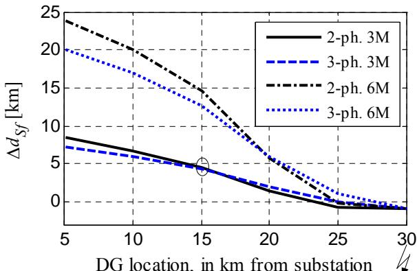
Fig. 2.  $\Delta d_{sf}$  for faults at the end of the feeder, on the main branch. There is one DG-unit, and the connection point is varied. Low load.
