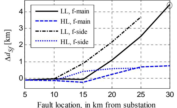
Fig. 3.  $\Delta d_{sf}$  with the DG connected 15 km from the substation on the main branch, and the fault location is varied. All faults are 2-phase short-circuits.
