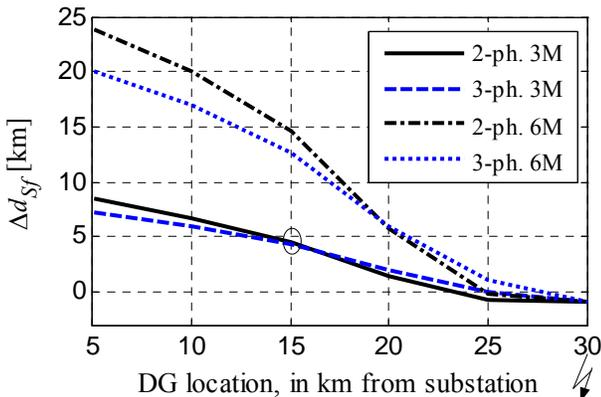
Fig. 2.  $\Delta d_{sf}$  for faults at the end of the feeder, on the main branch. There is one DG-unit, and the connection point is varied. Low load.
