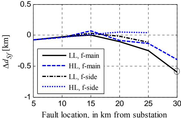
Fig. 10.  $\Delta d_{sf}$  with compensation A. The DG is connected 15 km from the substation. The faults are 2-phase short-circuits at varying locations.
