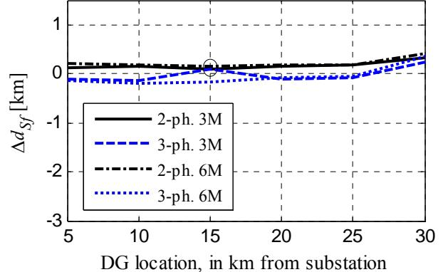
Fig. 11.  $\Delta d_{sf}$  with compensation B. All faults are at the end of the feeder, while the connection point of the DG is varied. Low load.
