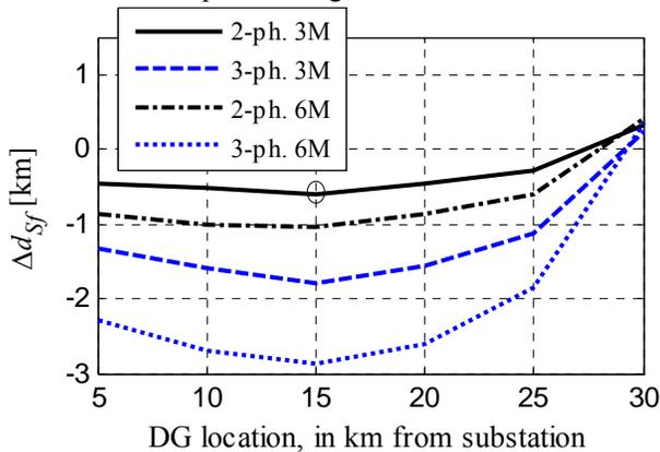
Fig. 9.  $\Delta d_{sf}$  with compensation A. All faults are at the end of the feeder, while the connection point of the DG is varied. Low load.
