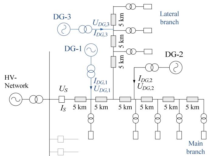
Fig. 1. Radial feeder with DG
