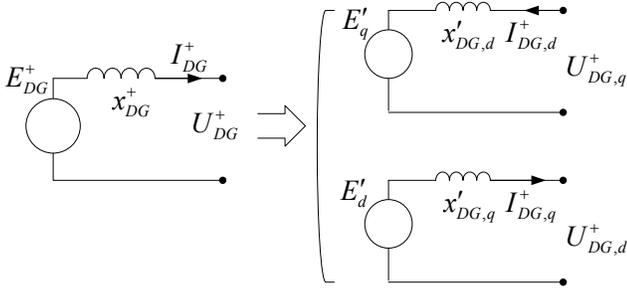
Fig. 7. Positive sequence equivalent circuit for the transient state
