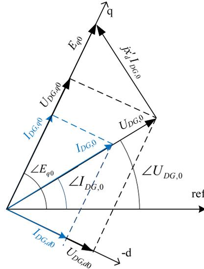
Fig. 6. Phasor-diagram for the DG-unit, in the pre-fault state
