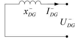
Fig. 8. Negative sequence equivalent circuit for the transient state
