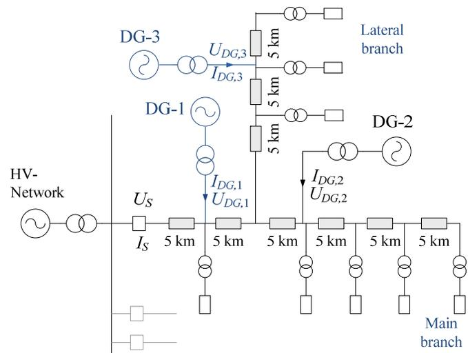
Fig. 1. Radial feeder with DG
