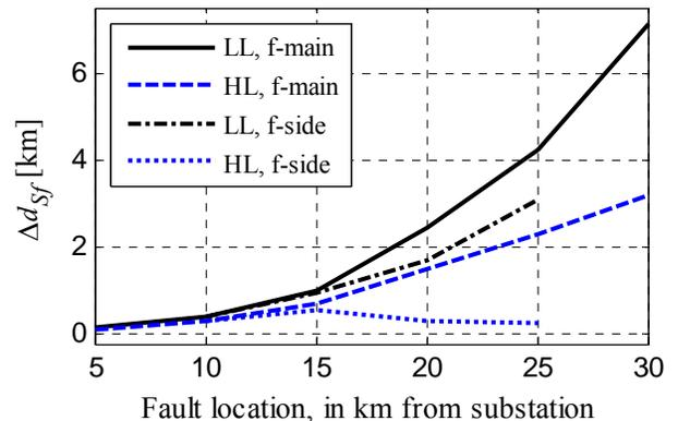
Fig. 4.  $\Delta d_{sf}$  with 3 DG units, generating 1 MW each, and the fault location is varied. All faults are 2-phase short-circuits.
