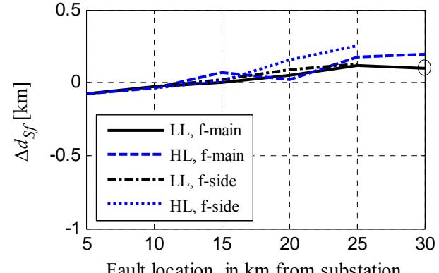
Fig. 12.  $\Delta d_{sf}$  with compensation B. The DG is connected 15 km from the substation. The faults are 2-phase short-circuits at varying locations.
