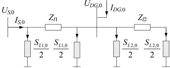
Fig. 5. Simplified representation of the feeder for analytical study. Loads are included as shunts in two pi-equivalents.
