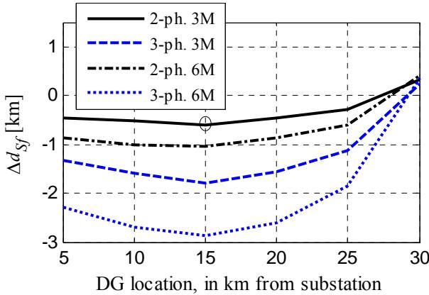
Fig. 9.  $\Delta d_{sf}$  with compensation A. All faults are at the end of the feeder, while the connection point of the DG is varied. Low load.
