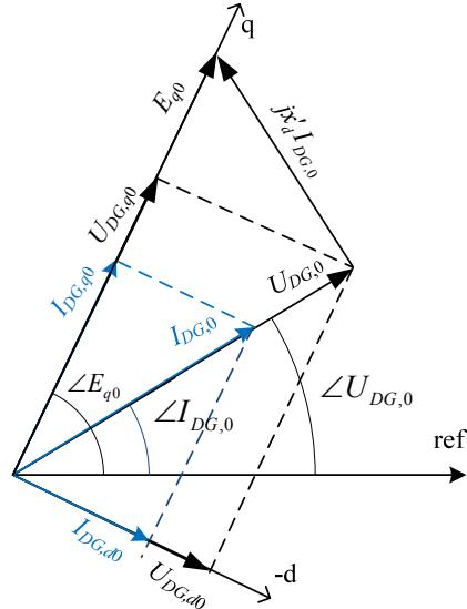
Fig. 6. Phasor-diagram for the DG-unit, in the pre-fault state
