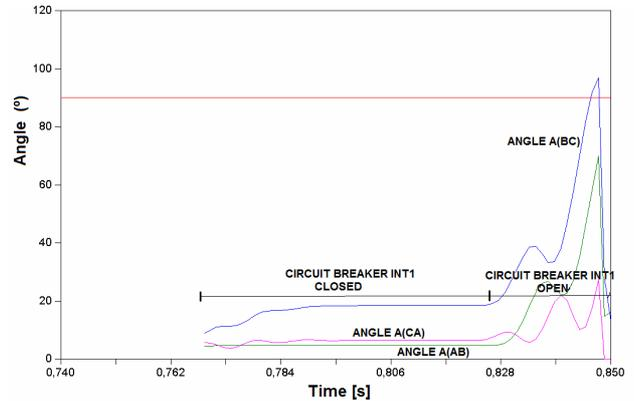
Fig. 13. Angle A for each DLP2 phase distance function
