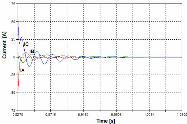
Fig. 12. Phase currents at Tacuarembó bus bar
