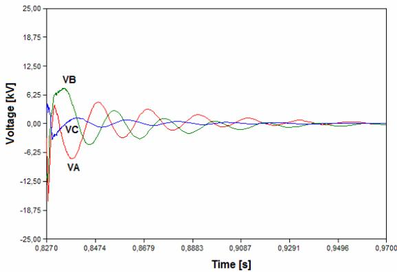
Fig. 11. Line to ground voltages at Tacuarembó bus bar
