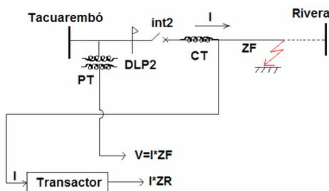
Fig. 5. Voltage and current supplied to DLP2 relay
