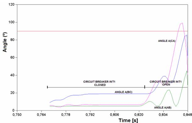
Fig. 16. Angle A for each DLP2 phase distance function
