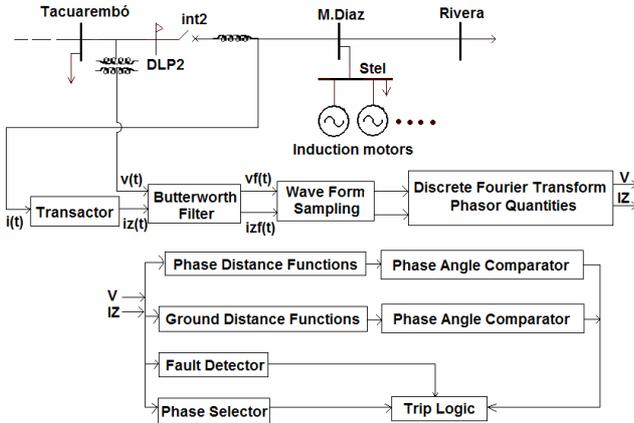
Fig. 2. Modules of ATP model
