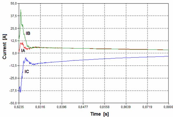
Fig. 15. Phase currents at Tacuarembó bus bar
