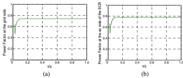
Fig.11 Power factor at the primary and the secondary side of the rectifier transformer without the application of the new SVC in system. (a) at the primary side. (b) at the secondary side.
