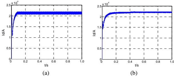
Fig. 5. DC currents of the new rectifier system with or without the new SVC. (a) without the new SVC. (b) with the new SVC.
