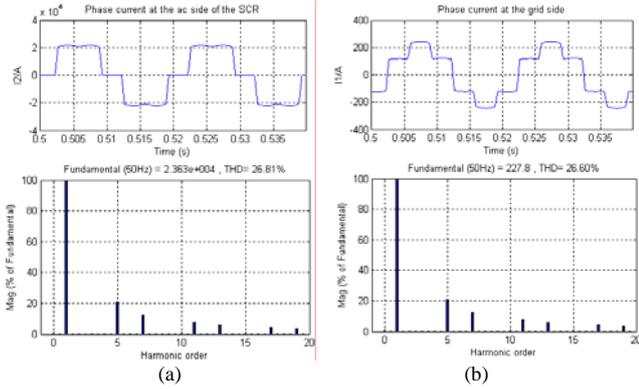
Fig.6. Phase current and its FFT at the secondary and the primary side of the new rectifier transformer without the new SVC in the system. (a) at the secondary side. (b) at the primary side.
