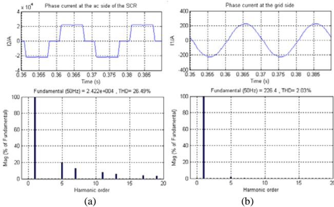
Fig.7. Phase current and its FFT at the secondary and the primary side of the new rectifier transformer with the new SVC in the system. (a) at the secondary side. (b) at the primary side.
