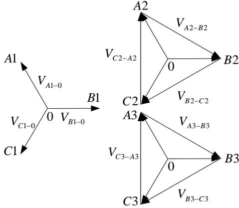
Fig.3. Voltage vector diagram of the new rectifier transformer
