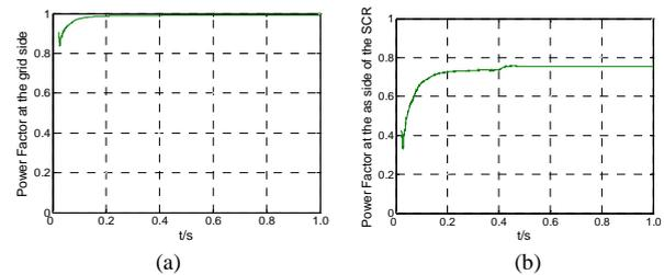
Fig.10 Power factor at the primary and the secondary side of the rectifier transformer with the application of the new SVC in system. (a) at the primary
