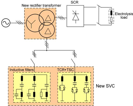
Fig.1. Main circuit topology of the new rectifier system with the new SVC
