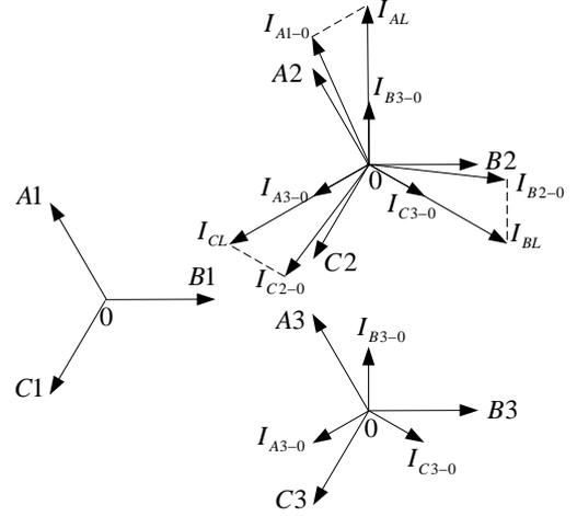
Fig.4. Reactive power compensation characteristic of the new SVC
