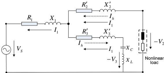
Fig.2. Single-phase equivalent circuit model of the new rectifier transformer
