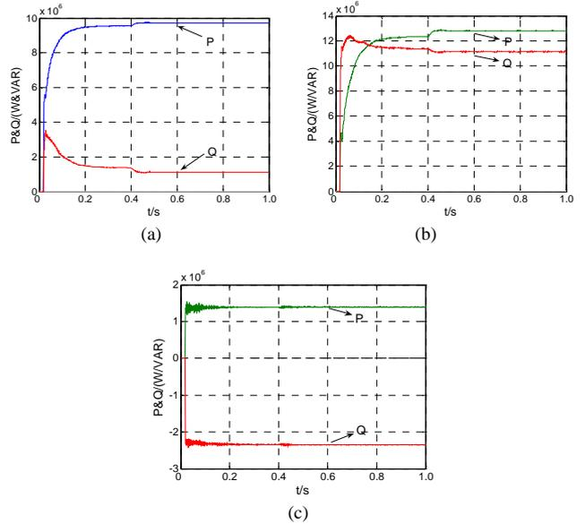
Fig.8. Active and reactive power (P&Q) at the primary, the secondary, and the third side of the new rectifier transformer with the application of the new SVC in system. (a) at the primary side. (b) at the secondary side. (c) at the third side.
