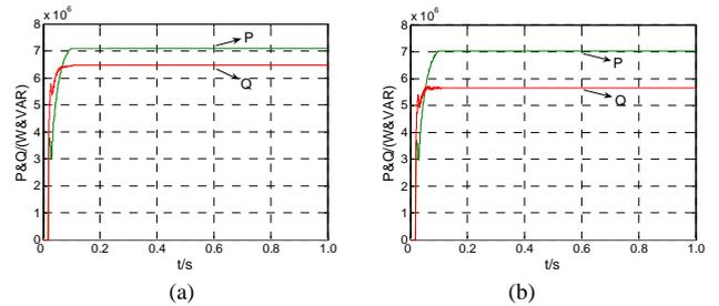
Fig.9. Active and reactive power (P&Q) at the primary and the secondary side of the new rectifier transformer without the application of the new SVC in system. (a) at the primary side. (b) at the secondary side.
