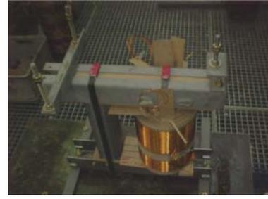
Figure 2. Test transformer under construction.
