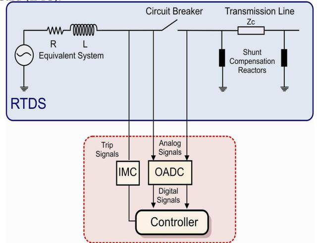
Fig. 4. Test setup with showing interfaced signals
