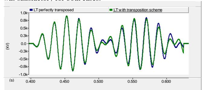
Figure 7: Comparison: LT perfectly transposed and LT with transposition scheme 1/6 - 1/3 - 1/3 - 1/6
