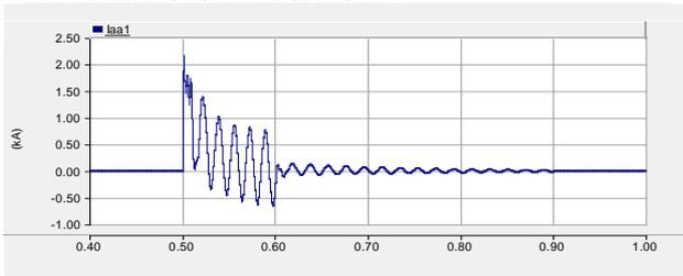
(a) Fault current. Phase A under fault.
