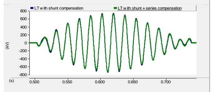
Figure 6: Comparison among shunt compensation TL vs. shunt+series compensation TL.
