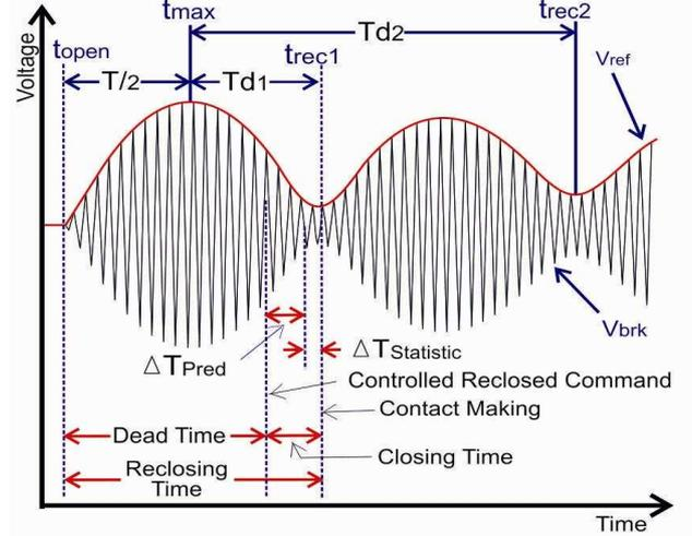
Fig. 3. Identification of optimum instants for TL reclosing
