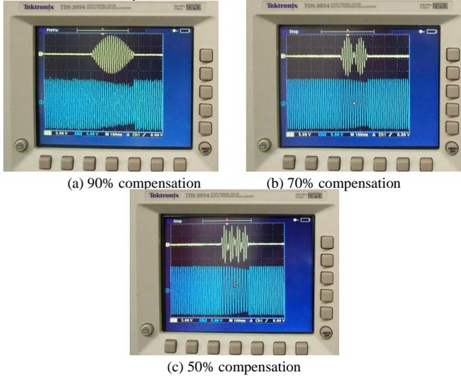
Fig. 5. Reclosing of TL using the developed controller.
