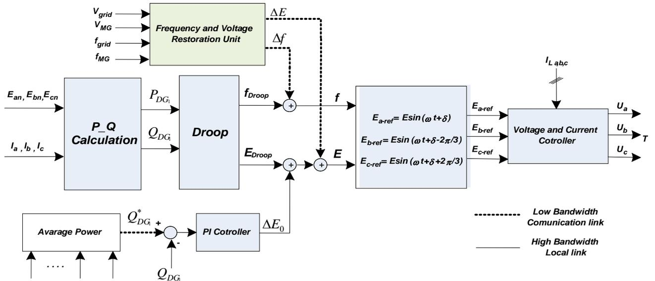
Fig. 1. The proposed scheme for accurate power sharing and frequency-voltage restoration.
