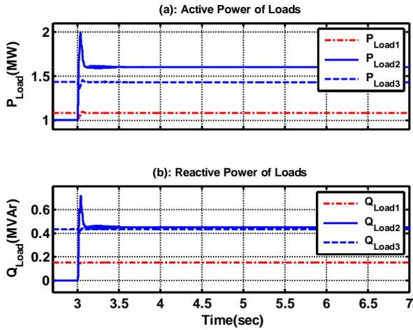
Fig. 3. A sudden load change in feeder 2. (a) Active power and (b) Reactive power of 20 kV feeders.
