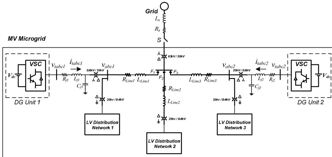
Fig. 2. A MV Microgrid consisting of two DGs
