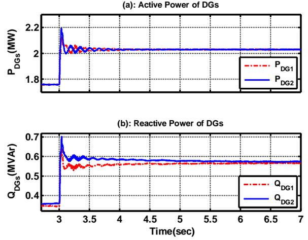
Fig. 6. The output power of DGs when a sudden load change is occurred in feeder 2 while the proposed method is used for power sharing. (a) Real power, (b) Reactive power of DGs
