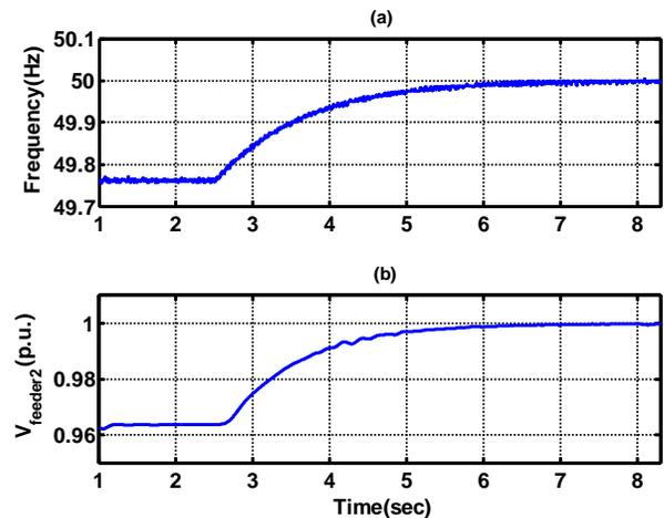
Fig. 9. Frequency and voltage restoration process of microgrid which start in  $t=2.5$ se. (a) Frequency of PCC, (b) Voltage of PCC
