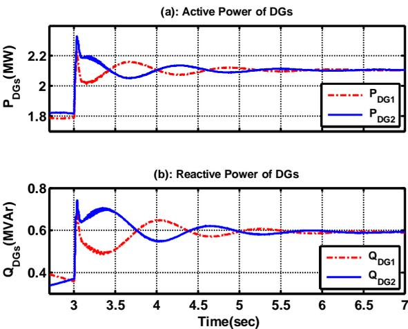
Fig. 5. The output power of DGs when a sudden load change is occurred in feeder 2 while APS method is used for power sharing. (a) Real power, (b) Reactive power of DGs
