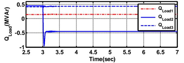
Fig. 7. Reactive power of 20kV feeders when a capacitor load switching is occurred in feeder 2.
