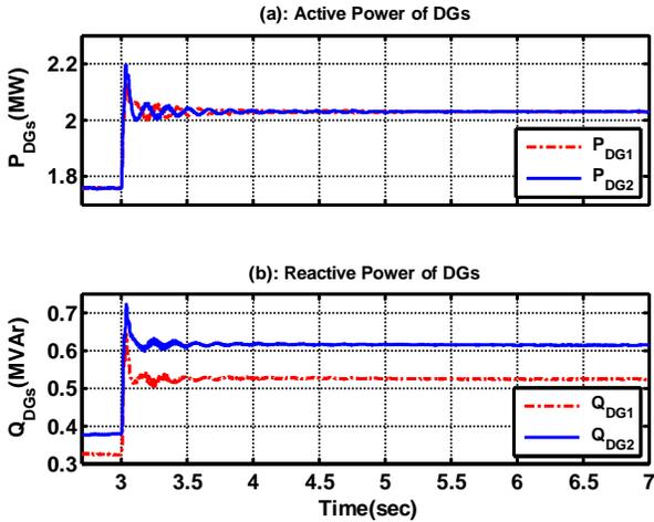
Fig. 4. The output power of DGs when a sudden load change is occurred in feeder 2 while the droop method is used for power sharing. (a) Real power, (b) Reactive power of DGs
