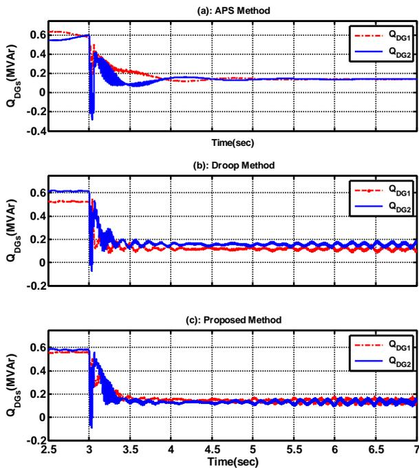
Fig. 8. The output power of DGs when a capacitor load switching is occurred in feeder 2 while (a) the droop method, (b) APS method and (c) proposed methods are used for power sharing.
